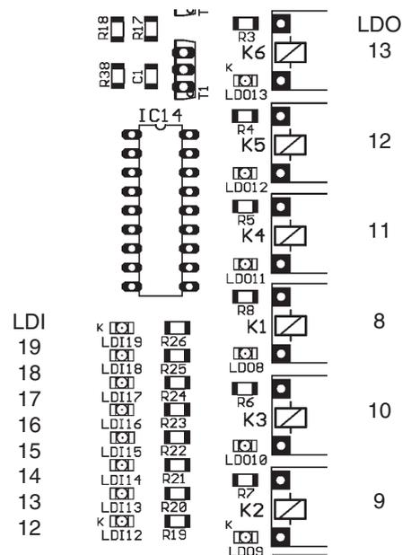
The EDIO-board is an expansion board for digital inputs and outputs. It can be attached to the I/O controller board at any of the four sockets and will be recognized by the IOC after a self test.
