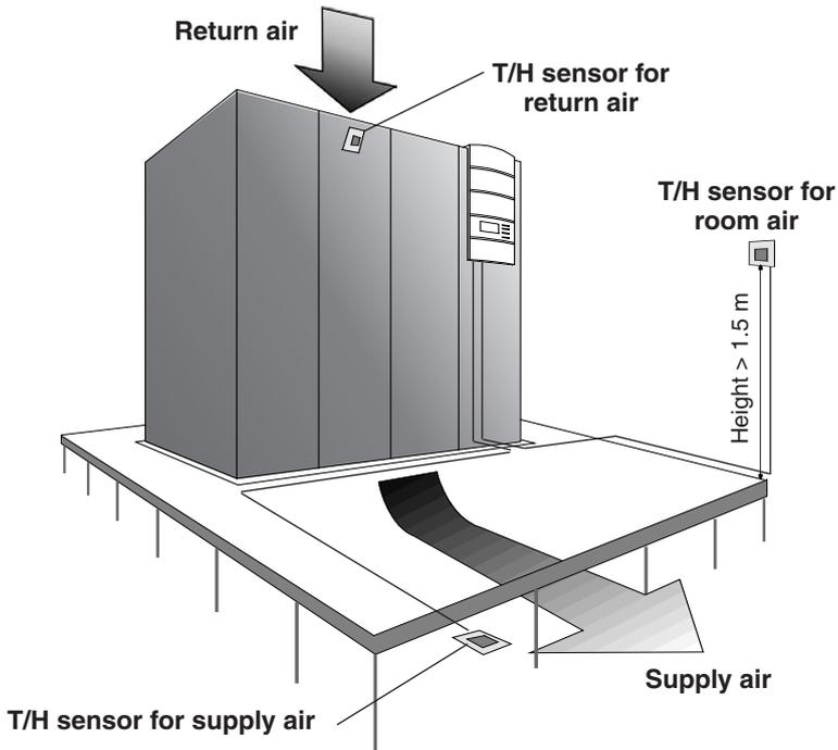
The sensor should be positioned depending on the room conditions, the thermal load distribution in the room and selected type of control. The maximum distance to the IOC can be 20m.
