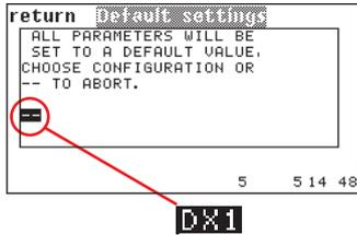
10 default configurations for different unit cooling systems are stored in the I/O controller.
