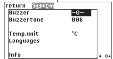
3. In the system menu, the alarm buzzer can be turned on (-1-) or off (-0-) and its pitch can be adjusted by selecting Buzzertone.
