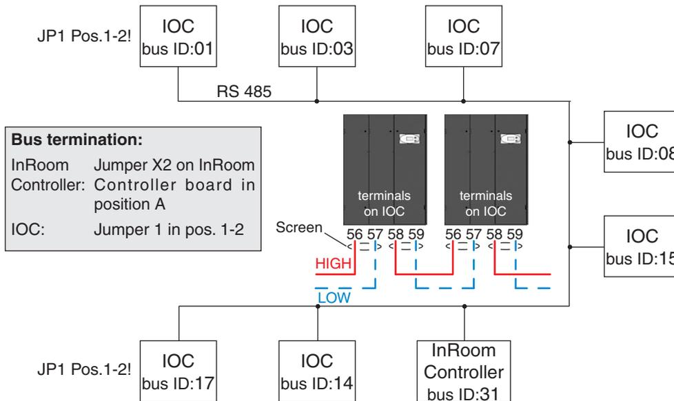
The bus address or bus ID is adjusted with the dip-switches on the IOC. The table at the right shows the corresponding adjustment for all possible bus IDs. The counting begins with 0 and ends with 31. A "1" means a dip-switch is in the ON position.
