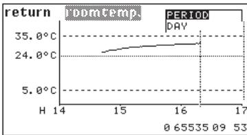
Use the data logger to save measured values or average values (zone data) calculated by the controller and have these values displayed in the shape of a graphical curve so as to show their time course.
