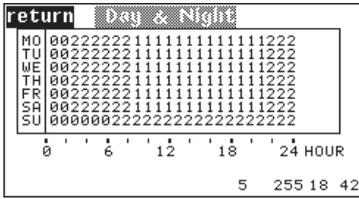
The week timer is based upon two different temperature setpoints which you have already adjusted in the control/temperature menu. Setpoint 1 is represented by a thick line, setpoint 2 by a dotted line. For each hour of each day of the week you choose among three settings:
