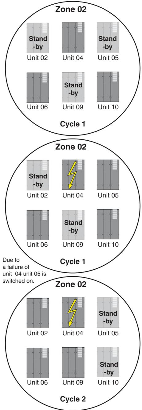
Due to a failure of unit 04 unit 05 is switched on.
