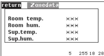
Here you can see the measured values for the zone. These values represent an average value for each parameter, which is calculated from all sensors of the units which are assigned to the same zone.
