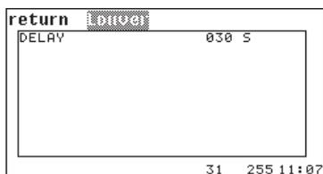
The pre-start serves to open the louver before the fan operation starts. This way a fan operation against a closed louver is avoided. ❶
