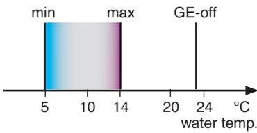
On the InRoom Controller you can adjust the water temperature limits for dehumidification here. However, this is also possible in the dehumidification menu.
