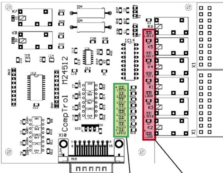
green LEDs for digital inputs 12-19 of the first EDIO-board
