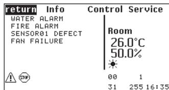
The alarm messages are displayed in the standard window of each unit with IOC. At the same time the symbol
