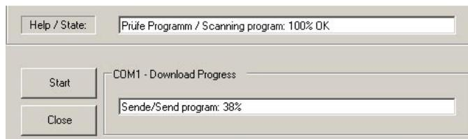
You can start the download by clicking the Start button. The single steps are indicated in the "Help/State" line, the progress of each step in the "Download Progress" line.
