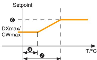
If the cooling unit has low airflow during nominal operation, the fan speed can be raised when the temperature setpoint is exceeded. The fan speed increase depends on the temperature difference to the setpoint.
