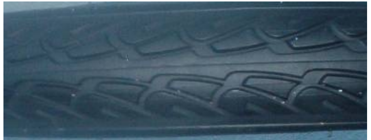
In the picture on the up, the “arrows” point left, giving you direction of rotation.
