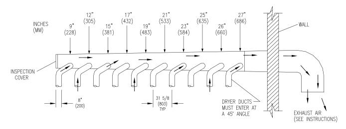
FIGURE 2- Dryer Exhausting Using A Main Discharge Duct.
