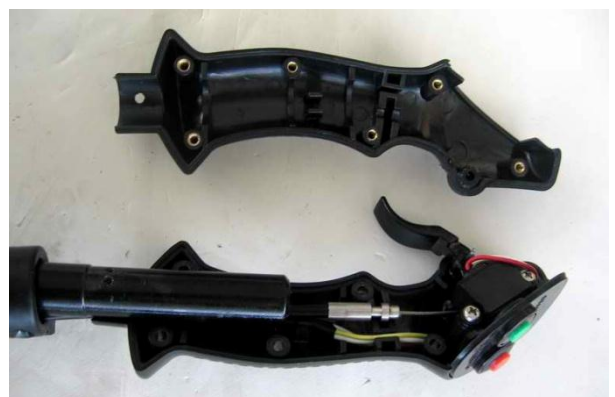
Throttle cable in joystick handle
