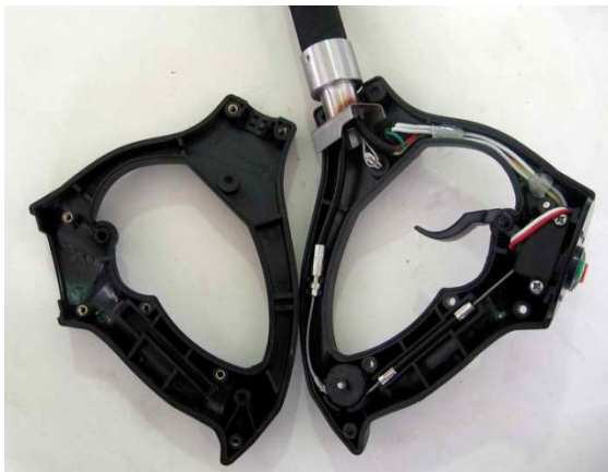
Throttle cable in Jetsurf handle
