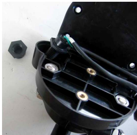
Jetkayak center control kill switch wiring
