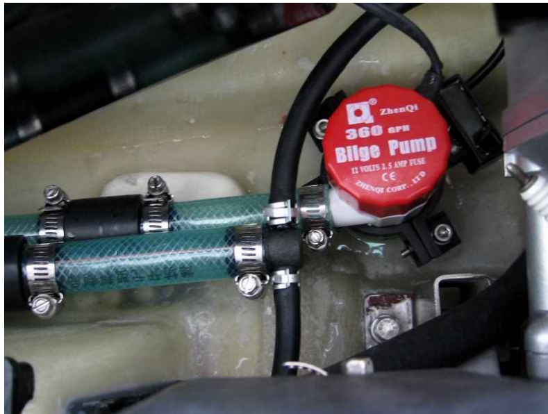
Bilge installed in engine compartment
