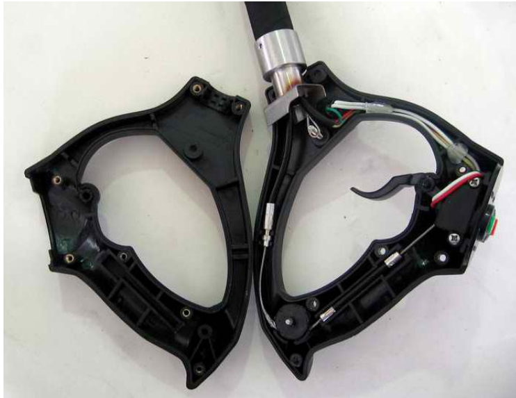
Jetsurf handle switches and wiring
