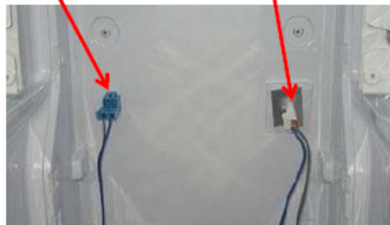
Defrost heater +temp. fuse housing
