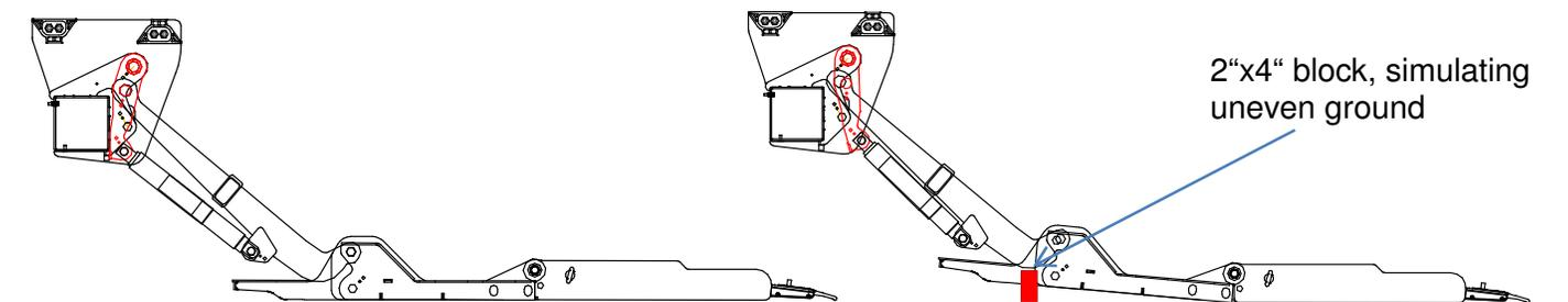
While swing arm is detaching from main frame lift cylinders keep retracting to compensate for rotation of platform. Platform stops lowering down when main section meets ground or cylinders are completely retracted.
