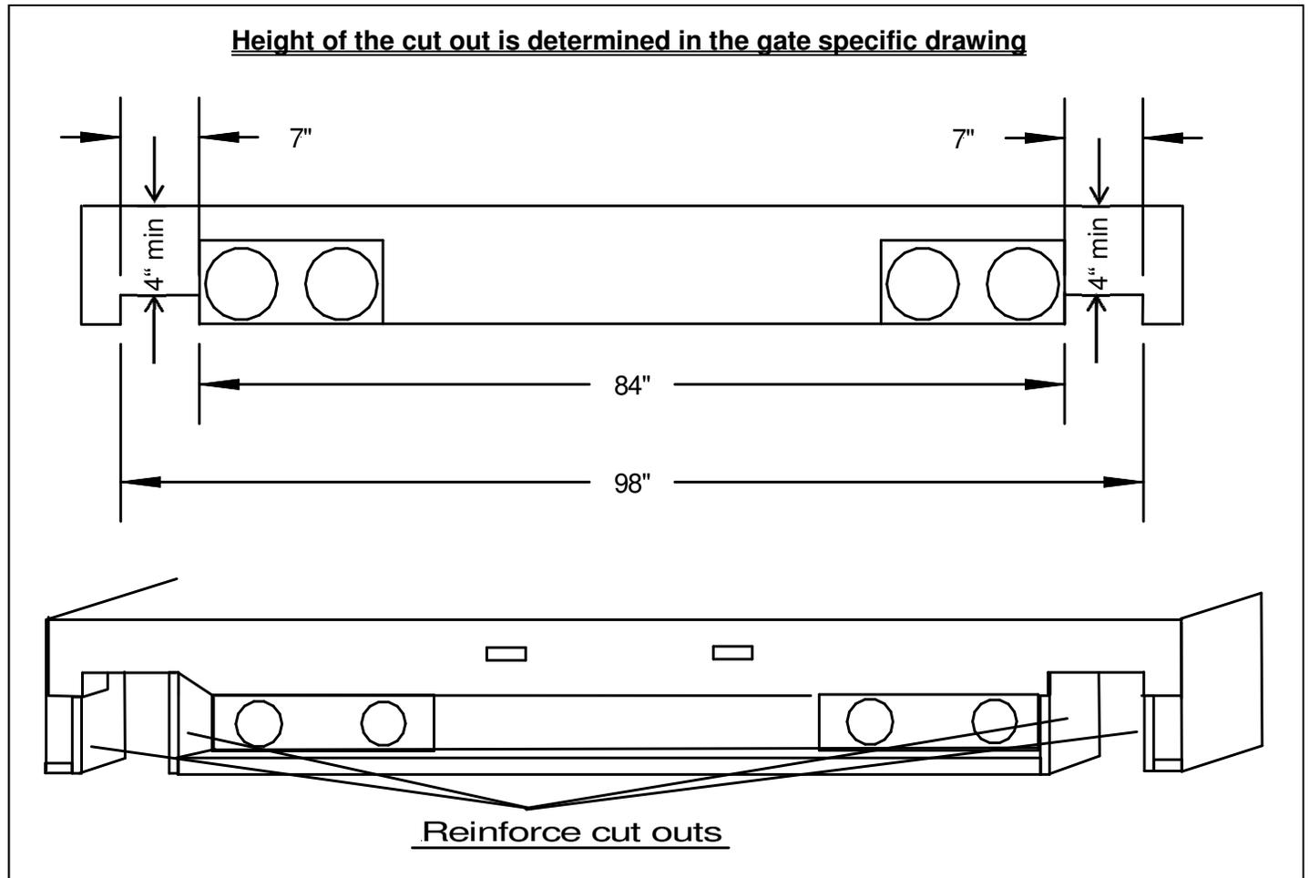
Figure 5 Sill cut-out dimensions - rear view
