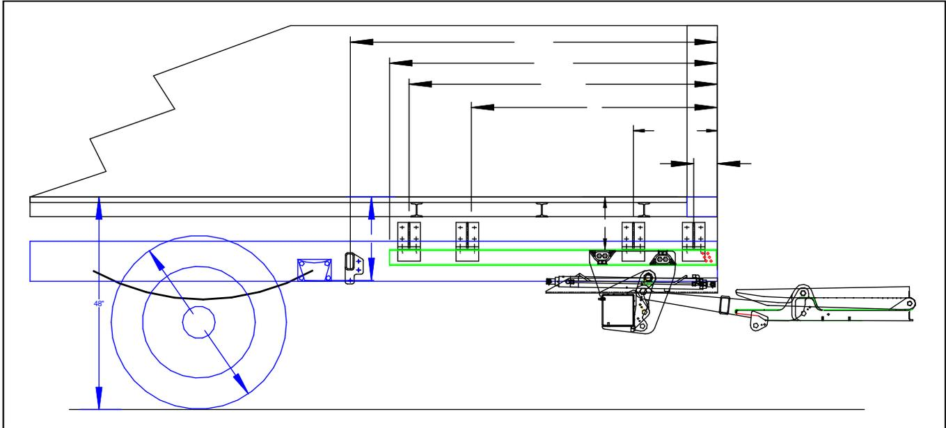
Figure 9 Liftgate installation to previous installed rails
