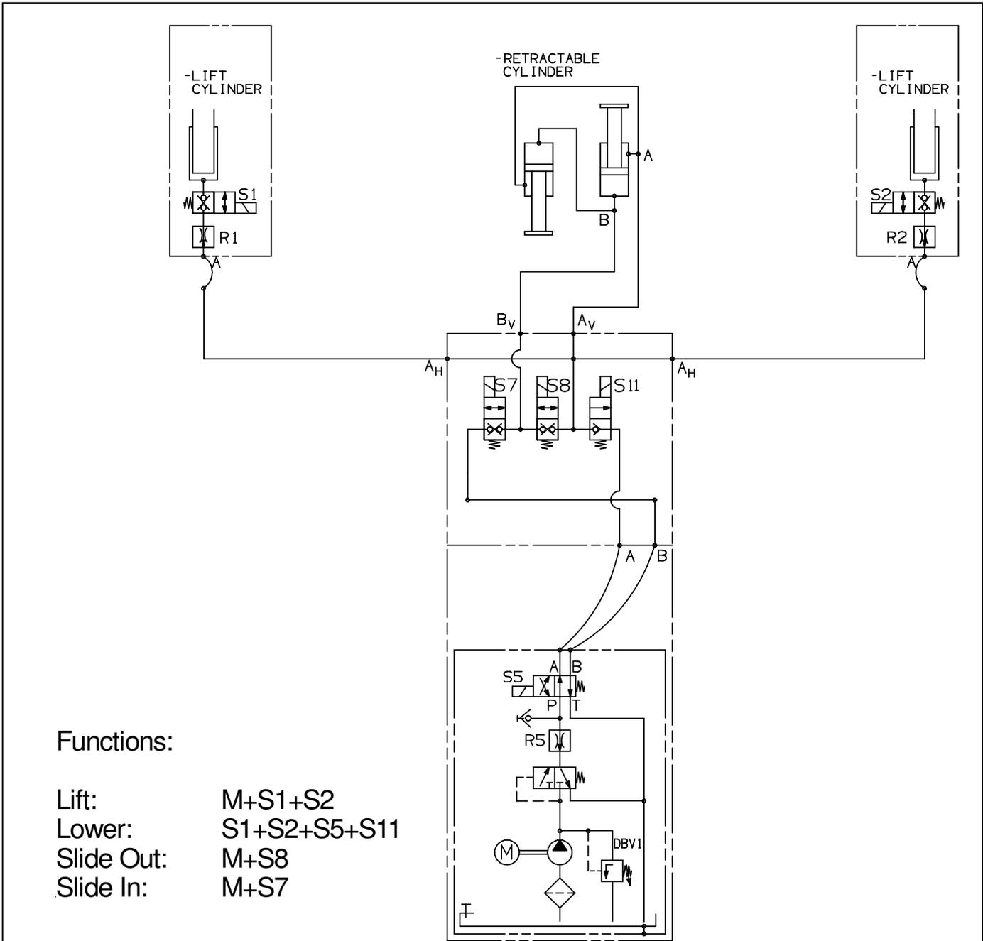
S1, S2 on lift cylinder and S7, S8 on push pull valve block are double acting release valves: They have to be activated for fluid to go through them in either direction
