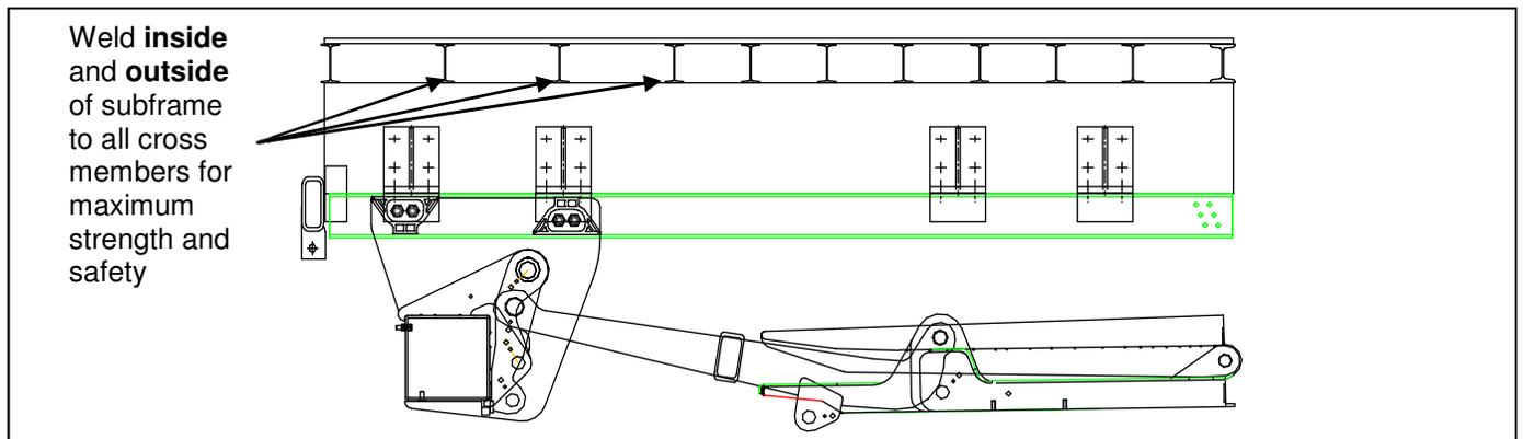
Figure 11 Quick mount weld-on setup
