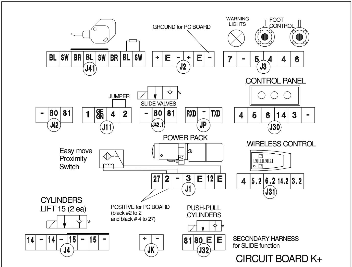
Figure 29 Plug setup on PC - Board
