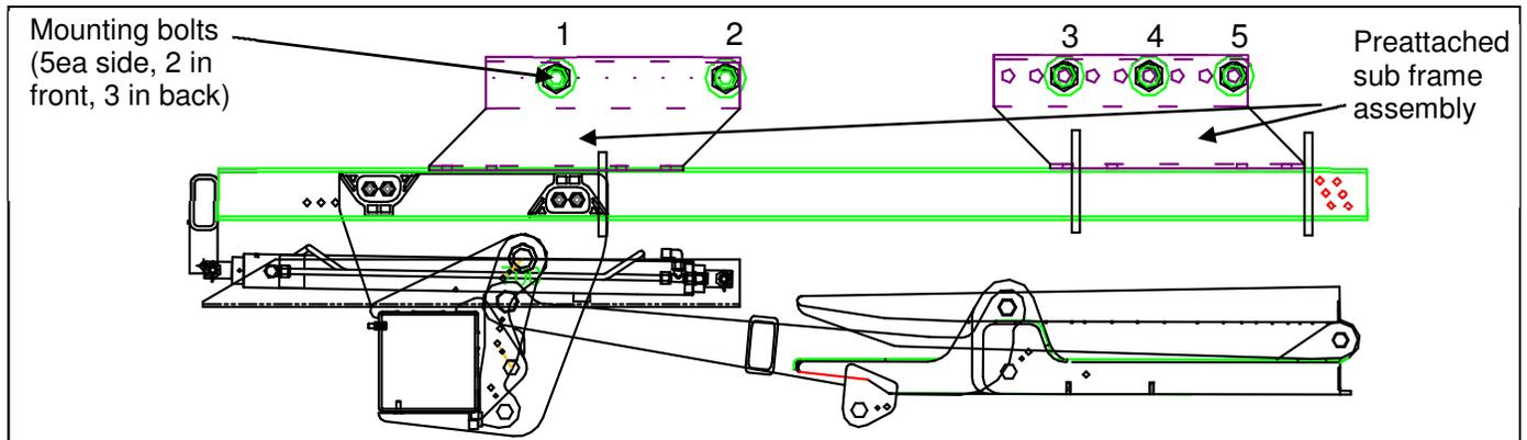
Figure 10 Rapid mount bolt-on setup
