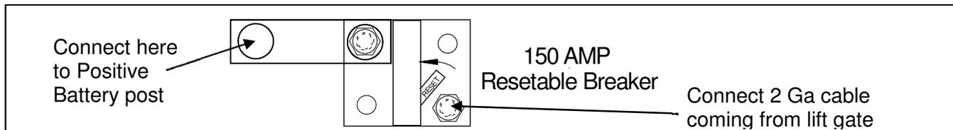
Figure 19 Circuit breaker installation
