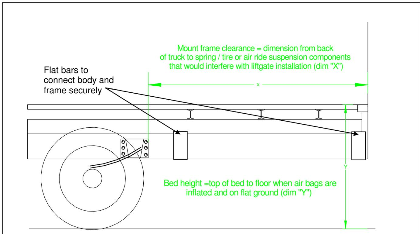
Figure 4 Mounting clearance
