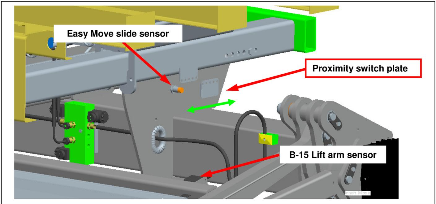
When successfully installed the ILFP, the **Easy Move option has to be activated**. In order to do that, proceed with the following steps:
