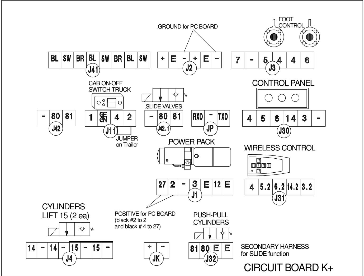
Figure 27 Plug setup on PC - Board
