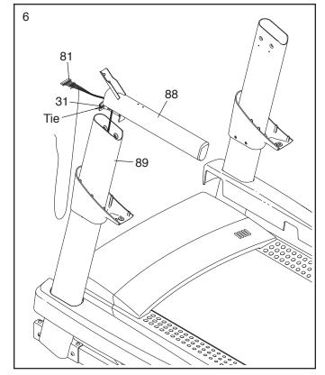
7. Attach the Left Handrail (88) to the Left Upright (89) with two 5/16" x 1" Screws (5), two 5/16" Star Washers (11), and a 5/16" x 1 1/4" Bolt (4). **Do not fully tighten the Screws and Bolt yet.**
