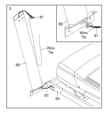
4. Hold the Left Upright (89) against the Base (94). Be careful not to pinch the Upright Wire (81). Insert two 3/8" x 1 1/4" Screws (8) with two 3/8" Star Washers (13) and two 3/8" x 2 3/4" Screws (7) into the Left Upright.
