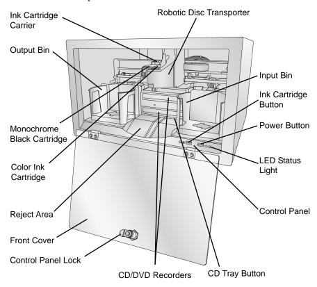
The Robotic Disc Transporter moves discs from the Input Bin, to a CD/DVD Recorder, to the printer, and finally to the Output Bin.
