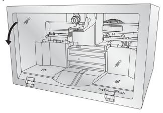
• The Publisher will automatically position the cartridge carrier and Robotic Disc Transporter to the center position allowing for easy access to the bins.
