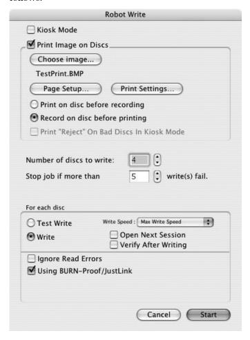
a. **Kiosk Mode** will allow you to increase the capacity of your Publisher from 50 to 100 discs by dispensing finished discs out the front of the unit instead of dropping them to the output bin. This allows you to place blank discs in both the input and output bins doubling your capacity.
