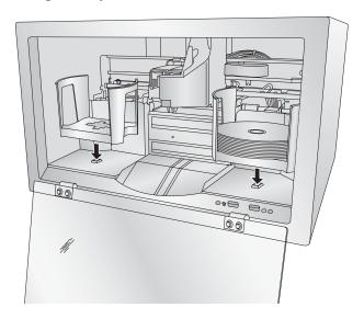
• Load the Input Bin (the bin located on the right-hand side of the Publisher) with 50 blank discs and place the bins on the mounting pegs.
