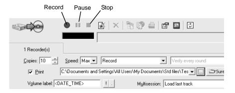
While jobs are running, they may be paused or stopped by clicking on the appropriate buttons on the Job Setup Panel. The Pause Button will allow the current recording to finish, then suspends operations on that job. Recording is resumed by clicking the Pause Button again.
