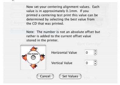
Look at the finished alignment disc and pick the numbers that come closest to lining up with one another. For instance, on the disc shown in this manual, the vertical alignment is 2 and the horizontal alignment is 0. Enter this in the alignment dialog box.
