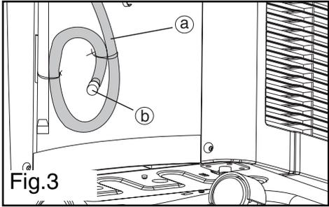
3. Route the end of the hose under the side of the water tank, then through the hole provided on the face of the tank and place the water tank back into the cabinet (As shown in Figure 4). *If required*, attach the included drain hose adapter (Fig 4) to the end of the drain tube and attach a section of garden hose (not included) to suit your continuous drain option requirements.
