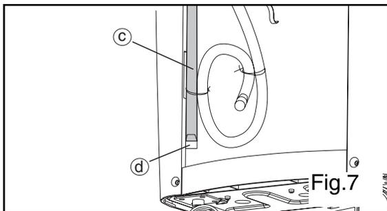
**CAUTION:** Failure to replace and recap the direct sump drain tube prior to using the unit may result in flooding of the immediate area.
