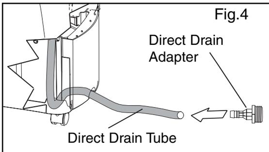
**Please Note:** Remember to reverse the above direct drain instructions when relocating the unit to a location where continuous drain is not possible. Failure to replace and recap the direct drain hose may result in flooding of the immediate area.
