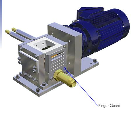
The finger guard on the Cold Jet AeRO 75 series protects from a potential personal injury site located inside the machine. The guard, over the air exhaust port, must remain installed at all times to serve its function.
