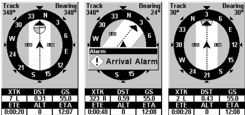
Navigate trail, navigation page (compass rose) views: at left, boater is northbound heading straight toward trail point 3; bearing arrow shows the trail point straight ahead. At right, driver has reached trail point 3 and must turn northeast to follow the trail. Arrival alarm goes off and bearing arrow swings around to say turn right (northeast), toward the next waypoint, trail point 4. The Cuda 240 now shows navigation information to point 4, which is 0.43 miles away.
