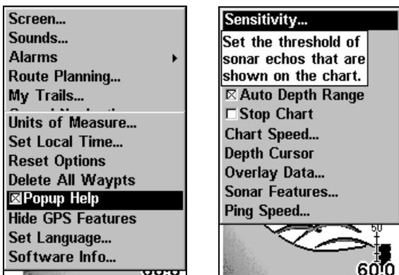
System Setup Menu, left, with Pop-up Help command highlighted. At right, this example shows the Pop-up Help message for the Sensitivity command, located on the Sonar Menu.
