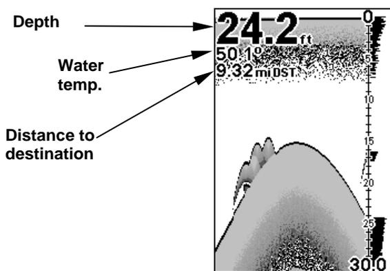
Sonar Page with Overlay Data turned on. This example shows Depth, Water Temp. and the Distance to the next waypoint in the current route.
