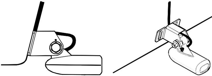
Route cable over bolt and through bracket. Side view shown at left and seen from above at right.
