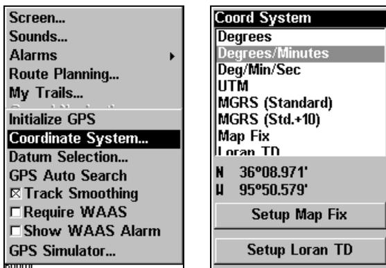
Menus for changing coordinate system used to display positions.
