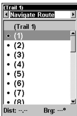
Navigate a trail menu sequence: Fig. 1, My Trails command. Fig. 2, Trails Menu. Fig. 3, Edit Trail Menu. Fig. 4, Edit Route Menu with Navigate command highlighted for Trail 1. A trail is always converted to a "route" when you navigate the trail.
