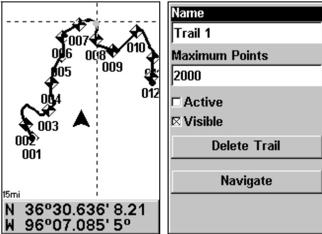
At left, trail selected with plotter cursor. The info box at the bottom of the screen shows distance and bearing from current position to the selected point on the trail. At right, the Edit Trail menu.
