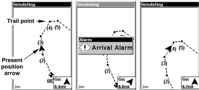
Navigate trail, plotter views: at left boater is heading straight toward trail point 3. Center, when the point is reached, Arrival Alarm goes off and the steering arrow points toward next trail point. At right, boater has reached point 3 and has turned northeast to follow trail to point 4. (Flashing trail line is turned off for clarity.)
