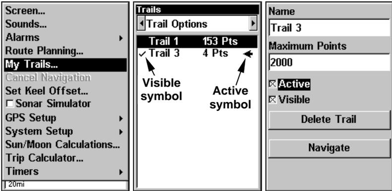
Sequence for saving a trail and beginning a new one. At left, My Trails command. Center, the Trails Menu. The arrow to the right of Trail 3 indicates the trail is "active," and the check to the left indicates the trail is visible on the plotter display. The right figure shows the Edit Trail menu, with the Active command selected.
