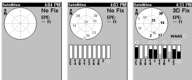
**Satellite Page.** Left view indicates unit has not locked on to any satellites and does not have a fix on its position. Center view shows satellites being scanned. Right view shows satellite lock-on with a 3D position acquired (latitude, longitude and altitude.)
