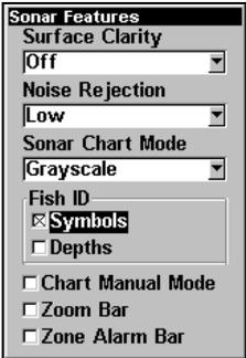
**Sonar Features menu with Fish I.D. Symbols selected. When the check box to the left is checked, the feature is on.**
