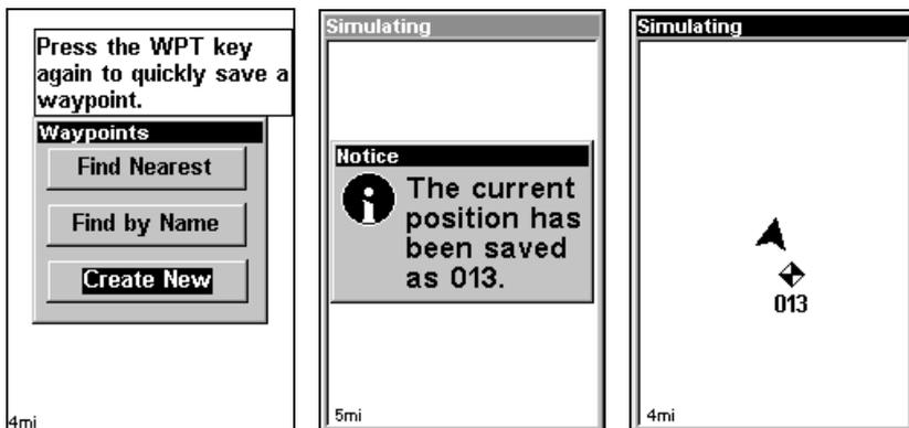
Sequence for setting a waypoint. Step 1: while traveling, *quickly* press **WPT twice** to call up Find Waypoint screen (shown at left) and set a point. Step 2: a message says the waypoint has been saved (shown center). Step 3: vehicle continues on its way; number waypoint symbol is visible on plotter (shown at right).
