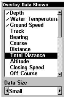
Data list showing "Ground Speed" turned on to display on Sonar Page.
