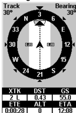
Navigating along a route: Figs. 1 & 4 show the Plotter Page (top) and Navigation Page (bottom) while running a route. Boater is heading straight for waypoint 3. In Figs. 2 & 5, the traveler has arrived at Wpt 3; the arrival alarm has been triggered and the bearing arrow on the compass rose has turned to point toward Wpt 4, off to the northeast. In Figs. 3 & 6 the traveler has turned northeast on his new course and is heading straight for Wpt 4, which is 0.43 miles away.
