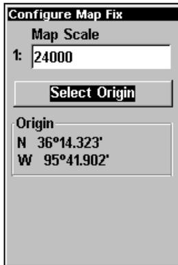
**Configure a map fix so the Cuda 240 can find your position on a printed chart or topographical map.**
