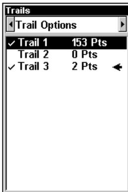
New trail, named "Trail 3," is created when Trail 2 is made inactive. Any new travel will be recorded in this trail, which is active and visible. Trails do not need to be visible in order to be active.
