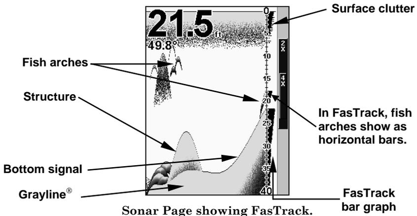
When the boat is not moving, fish signals are long, drawn out lines on a normal chart display. FasTrack converts the graph to a vertical bar graph that, with practice, makes a useful addition to fishing at a stationary location.
