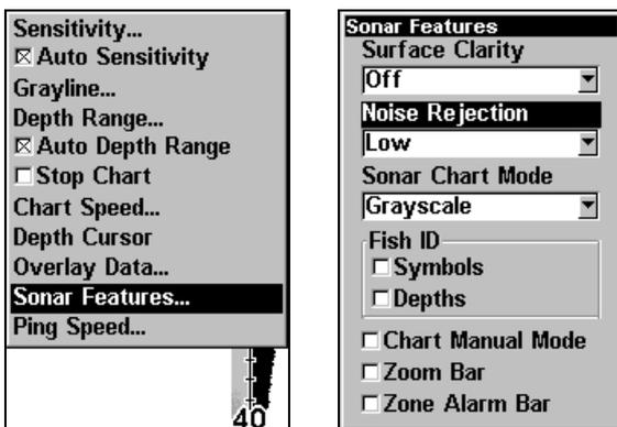
At left, Sonar Menu with Sonar Features selected. In the Sonar Features menu, Noise Rejection is selected with ASP in the default low setting.
