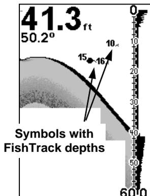
Sonar Features menu with Fish I.D. Depths selected. When the check box to the left is checked, the feature is on. At right, Sonar Page showing Fish I.D. symbols and FishTrack depths turned on.
