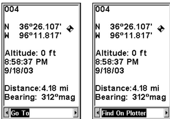
Waypoint information screen on waypoint 004. Screen shows name, latitude/longitude, distance to waypoint and its compass bearing. Figure at left shows **Go To** command; right figure shows **Find On Plotter** command.
