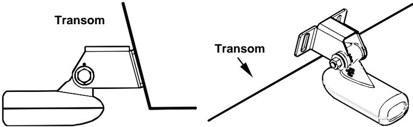
Position transducer mount on transom and mark mounting holes.
