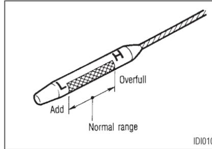
4. Remove the dipstick and wipe it clean. Reinsert it all the way.
