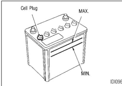
Check the fluid level in each cell (Remove the battery cover if it is necessary). It should be between the MAX. and MIN. lines.
