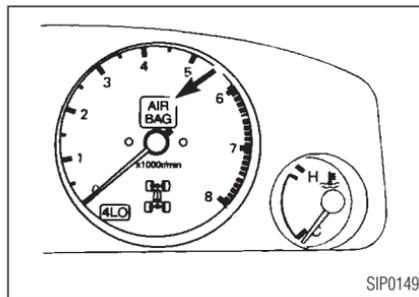
The supplemental air bag light, displaying “AIR BAG” in the instrument panel, monitors the circuits of the supplemental air bag. The circuits monitored by the supplemental air bag light are the diagnosis sensor unit, supplemental air bag modules and all related wiring.
