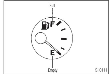
The gauge may move slightly during braking, turning, acceleration, or going up or down hill.
