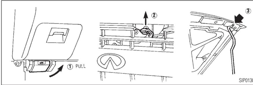
1. Pull the hood lock release handle located below the instrument panel; the hood will then spring up slightly.
