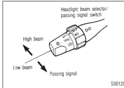
To select the high beam, push the lever for-
