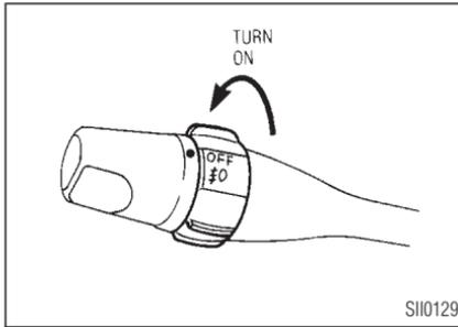
To turn the fog lights on, turn the headlight switch to the "☉" position, then turn the switch to the "☉" position. To turn them off, turn the switch to the "OFF" position.
