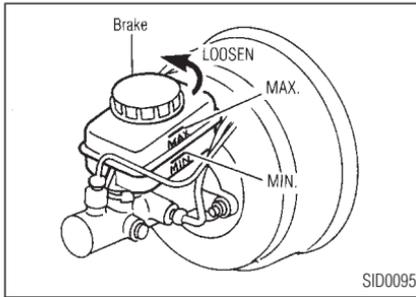
Check the fluid level in the reservoir. If the fluid is below the Min. line or the brake warning light comes on, add **DOT 3** fluid up to the Max. line. If fluid must be added
