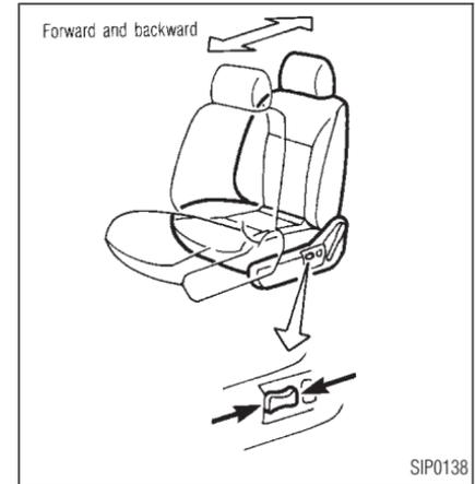
Pressing the switch forward or backward will slide the seat forward or backward to the desired position.
