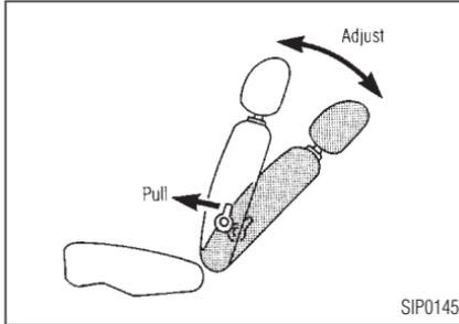
Pull the reclining lever and position the seatback at the desired angle. Release the reclining lever after positioning the seatback at the desired angle.
