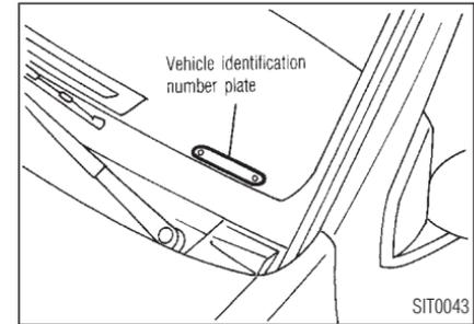
The vehicle identification number plate is attached as shown. This number is the identification for your vehicle and is used in the vehicle registration.
