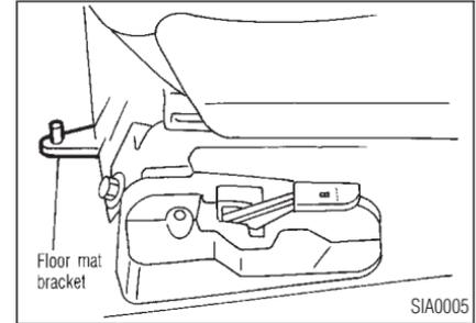
This model includes a front floor mat bracket to act as a floor mat positioning aid. INFINITI floor mats have been specially designed for your vehicle model. The driver side floor mat has a grommet hole incorporated in it. Simply position the mat by placing the floor mat bracket hook through the floor mat grommet hole while centering the mat in the floorpan contour.
