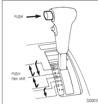
Push the button to shift into "P", or from "N" to "R", "P" to "R" and "D" to "2". All other positions can be selected without pushing the button.
