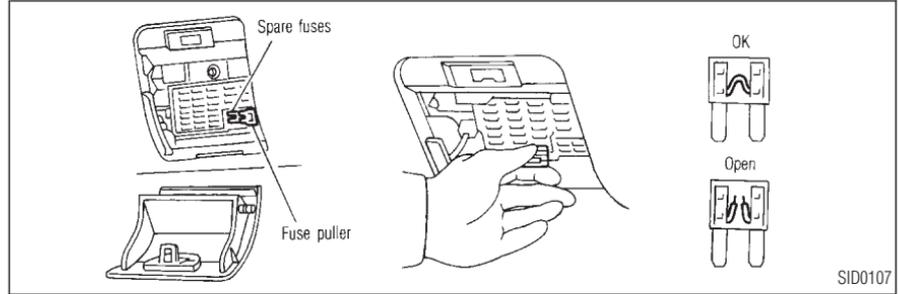
If any electrical equipment does not operate, check for an open fuse.
