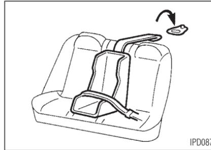
If your child restraint has a top strap, install the anchor bracket to the provided anchor point.
