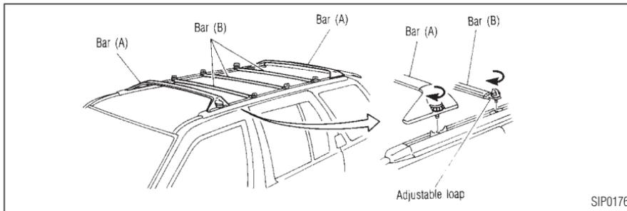
The cross-bars can be adjusted forward and backward. Place your luggage between the bars (A), adjust the bars (A), and secure the luggage with rope to the bars (A). There are also adjustable loops on the side bars for the rope attachment.
