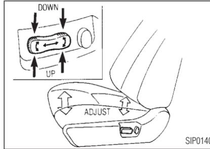
Pull or lower either side of the switch to adjust the seat cushion to the desired angle and height.
