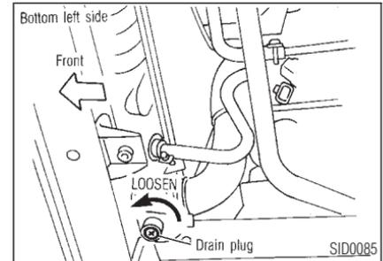
2. Open the radiator drain plug and radiator cap.
