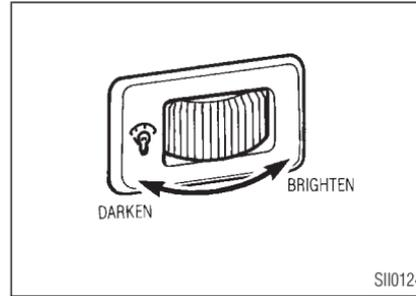
The instrument brightness control operates when the head light switch is in the "☉" or "☉" position.
