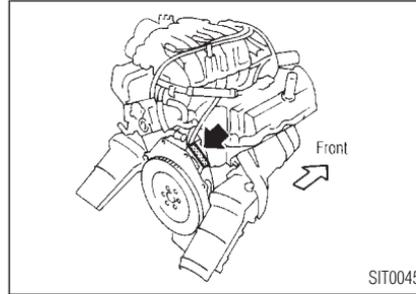
The number is stamped on the engine as shown.
