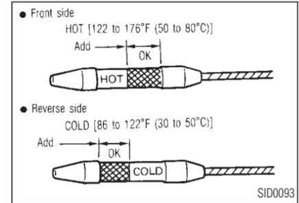
3. Check the fluid level with the engine idling.
