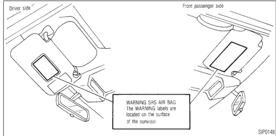
The warning labels about the supplemental air bag system are placed in the vehicle.
