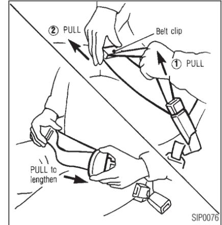
2. To lengthen, hold the tongue at a right angle to the belt and pull on the belt.
