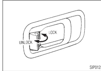
To lock from the outside without a key, move the inside lock knob to the "LOCK" position. Then close the door.
