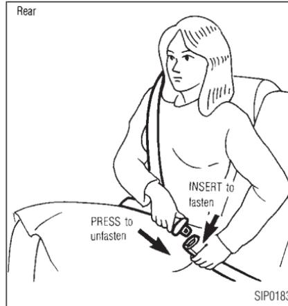
**The retractor is designed to lock during a sudden stop or on impact. A slow pulling motion will permit the belt to move, and allow you some freedom of movement in the seat.**
