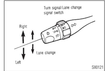
Move the lever up or down to signal the turning direction. When the turn is completed, the turn signals cancel automatically.
