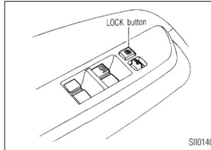
The passenger side switch will open or close only the corresponding window. To open or close the window, hold the switch down or up.
