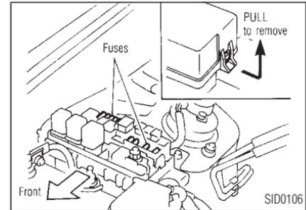
If any electrical equipment does not operate,
