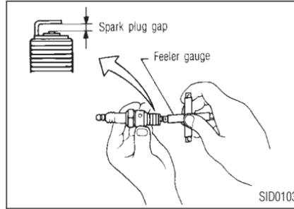
3. Check each new spark plug gap with a feeler gauge. Correct it as required.
