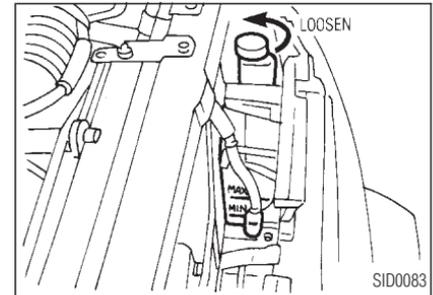
Check the coolant level in the reservoir tank when the engine is cold. If the coolant level is below “MIN”, add coolant up to the “MAX” level. If the reservoir tank is empty, check the
