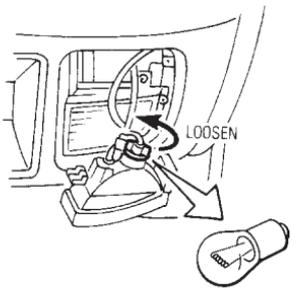
\* Remove after removing front turn signal light.
