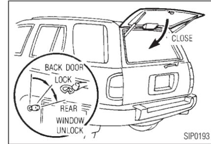
To open the rear window, turn the key fully clockwise and pull the handle. To close, lower and push the rear window down securely.
