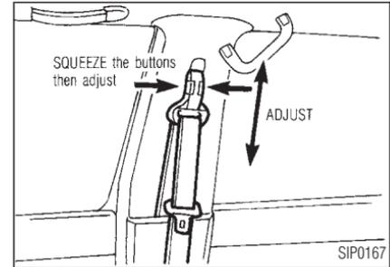
To adjust, squeeze the release buttons, and then move it to the desired position, so that the belt passes over the center of the shoulder. The belt should be away from your face and neck, but not falling off of your shoulder.
