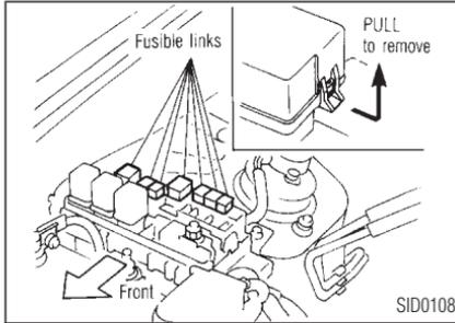
If any electrical equipment does not operate and fuses are in good condition, check the fusible links. If any of these fusible links are melted, replace only with genuine parts. See your INFINITI dealer.
