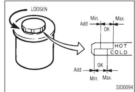
The fluid level should be checked using the "HOT" range on the dipstick at fluid temperature of 122 to 176°F (50 to 80°C) or using the "COLD" range on the dipstick at fluid temperature of 32 to 86°F (0 to 30°C).
