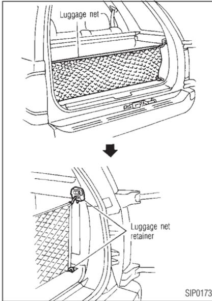
To install the luggage net, attach the four hooks to the four retainers.
