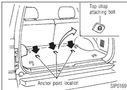
Anchor point attaching bolts are located under the carpet of the rear luggage area floor.
