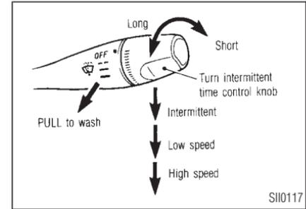
The windshield wiper and washer operates when the ignition key is in the “ACC” or “ON” position.
