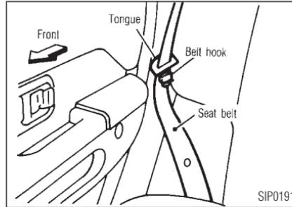
When the rear seat belt is not in use, hook it at the belt hook.
