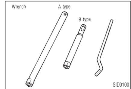
2. Remove spark plugs with a spark plug wrench. (Type A or B)
