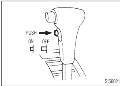
**ON:** For normal driving, push the overdrive switch “ON
