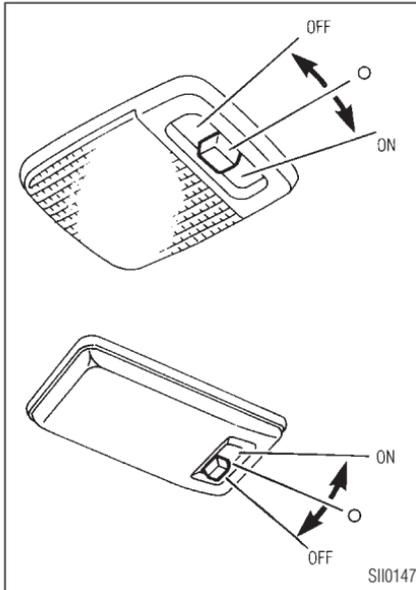
The interior light has a three-position switch.
