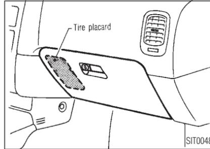
The cold tire pressure is shown on the tire placard affixed to the glove box lid.
