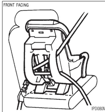
3. Pull on the shoulder belt until all of the belt is fully extended and a click is heard. At this time, the belt retractor is in the
