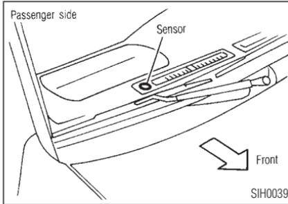
The sensor on the instrument panel helps maintain a constant temperature. Do not put anything on or around this sensor.
