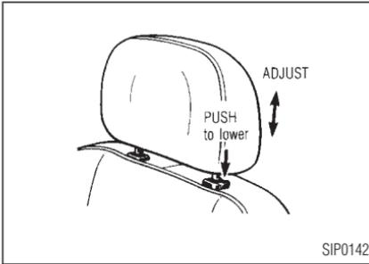
To raise the head restraint, just pull it up. To lower, push the lock knob and push the head restraint down.
