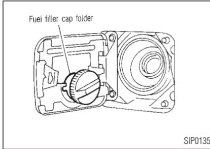
Put the fuel filler cap on the cap holder while refueling.
