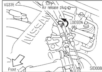
4. Flush the cooling system by running fresh water through the radiator.
