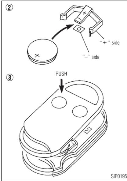
2. Replace the battery with a new one. Insert the battery as illustrated above.
