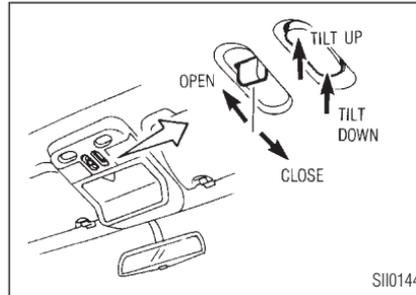
To open the roof, keep pressing the switch to the "←" side.
