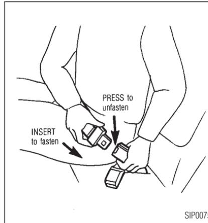
1. Insert the tongue into the buckle marked CENTER until it snaps.
