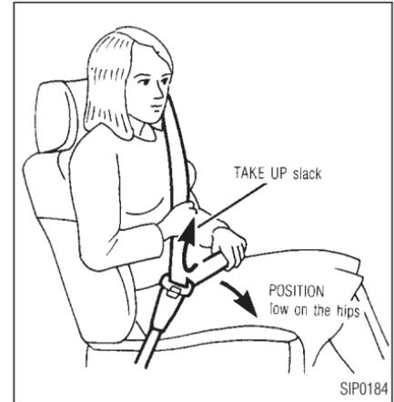
3. Position the lap belt portion **low and snug on the hips** as shown.
