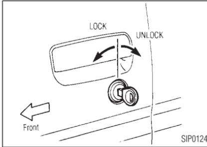
To lock the door, turn the key toward the front of the vehicle.
