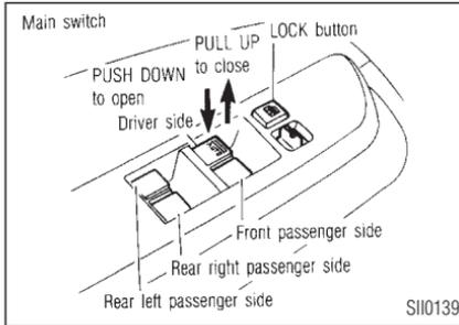
To open or close the window, push down or pull up the switch and hold it. The main switch (driver side switches) will open or close all the windows.
