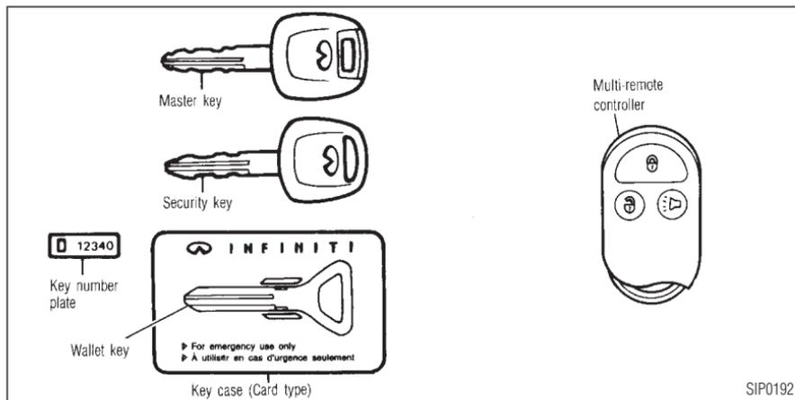
The master key and wallet key can be used for all the locks. The security key cannot be used for the glove box lock. To protect belongings when you leave a key with someone, give them the security key only. **Never leave this key in the vehicle.**
