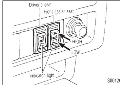
The front seats are warmed by built-in heaters. The switches located on the instrument panel can be operated independently of each other.
