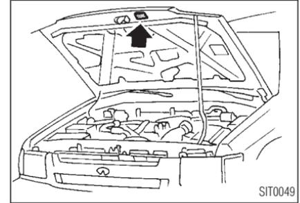
The air conditioner specification label is attached as shown.
