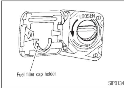
The fuel filler cap is a screw-on ratcheting type. Tighten the cap clockwise until ratcheting clicks are heard.
