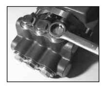
1. With a 27mm wrench, remove the three discharge plugs (#48) and three inlet plugs (#42A) from the manifold (#43).
