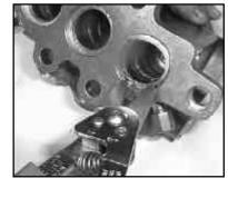
34. Install the rear support ring (#41), rear v-sleeve (#40), rear pressure ring (#39). Install the snap ring (#36).
