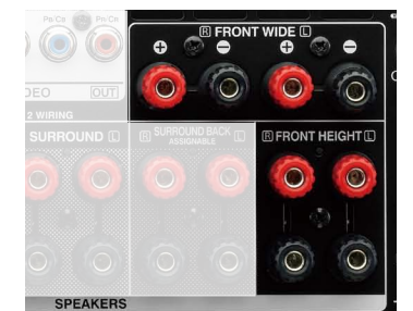
Front wide and front height special speaker terminals
