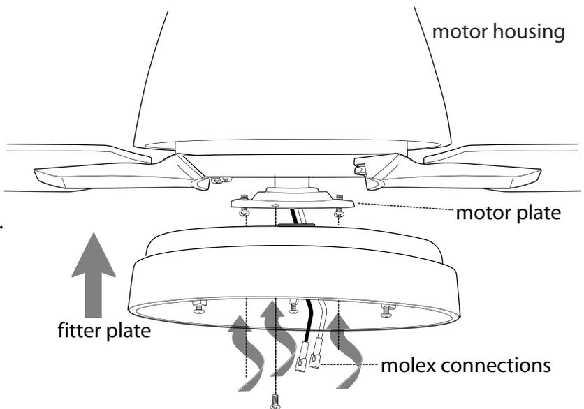
Remove 1 screw from post located on underside of fitter plate and partially loosen the other screws in the other two posts.
