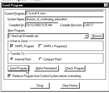
4. To verify that the program has been transferred successfully, select **Diagnostics** | **Report Program Information**. This should display a window that provides details about the current program loaded into the control system.
