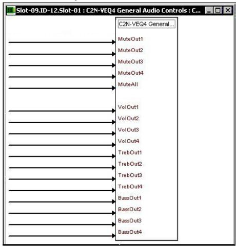
The C2N-VEQ4 symbol is defined by the assigned inputs. The diagram above shows the C2N-VEQ4 symbol in SIMPL Windows.
