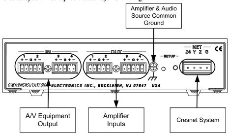
Four balanced/unbalanced inputs are provided for audio input, utilizing five-position mini-connectors. Audio inputs may be balanced using (+) and (-) inputs, or unbalanced using (+) input for signal and connecting (-) input to (G) and signal source ground.
