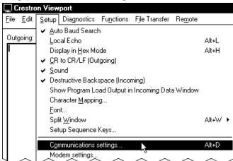
4. Select **RS-232** as the connection type. Verify that an available COM port (COM 1 is shown after this step) is selected, and that all communication parameters and necessary options from the "Port Settings" window are selected as shown on the next page. Click the **OK** button to save the settings and close the window.
