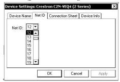
**NOTE:** SIMPL Windows automatically changes Net ID values of a device added to a program if a duplicate device or a device with the same default Net ID already exists in the program. Always ensure that the hardware and software settings of the Net ID match. For Net ID hardware setting details, refer to "Identity Code" on page 8.
