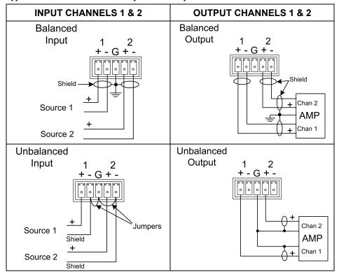
**NOTE:** Using the unbalanced configuration for the audio output reduces the total audio gain by  $6~\mathrm{dB}$ .
