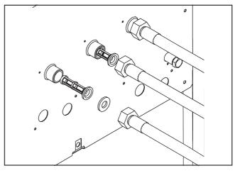
Check and clean regularly the filters in the water intake faucets, and the water intake hoses.
