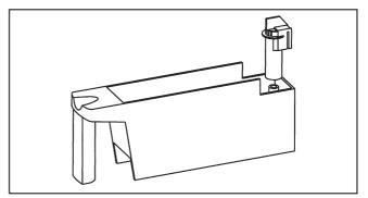
Pull the siphon tube out, clean it with warm water and reinsert it.
