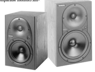
nels in existing HR824 front left/right systems or as a main monitor system in control rooms and editing suites where space is at a premium. When using the HR624 as the primary monitor in project rooms or off-line editing suites, mixes will flawlessly transfer to an "A" room that employs HR824's. The HR624 is flat ±1dB from 55Hz to 20kHz.
