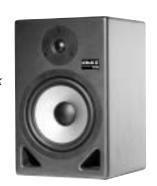
medium-density fiberboard construction to control sound reflection and standing waves within the monitor. Double-layer anodized aluminum cone offer extremely low distortion. Carefully molded woofer beauty rings improve midrange frequencies, while advanced dual-port tube designs create improved air flow for rich, solid bass response. Standard magnetic shielding makes placement easy in any studio environment.
