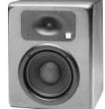
◆ Adjustments include level calibration and fine tuning of levels with a variable level control. XLR and RCA inputs accommodate balanced and unbalanced signals. The frequency response of bass and treble amplitudes can also be adjusted to compensate for placement and room absorption characteristics.
