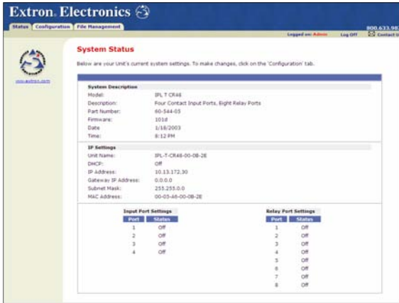
Figure 4-3 — Web server system status screen
