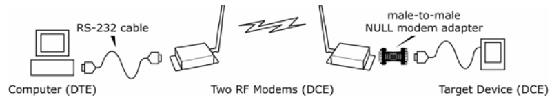
Figure B.3. Example of a MaxStream Radio Modem (DCE Device) connecting to another DCE device
