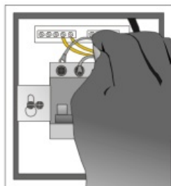
2. Put cables of three cores, 6mm 2 in the input of RCD
