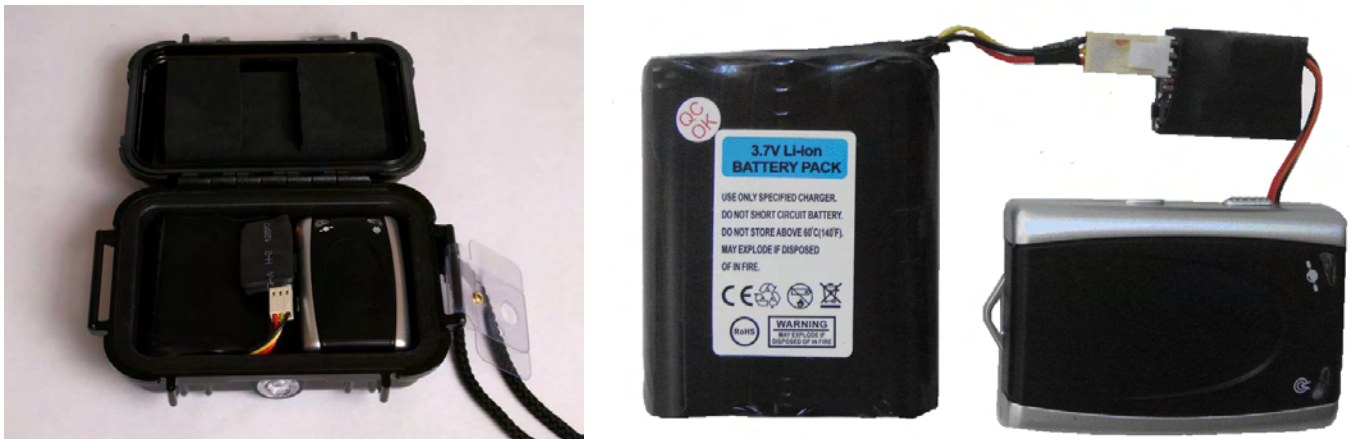
Fig 1: 6600mAh Battery with RT-99 and GC-101 GPS Tracker in Pelican GPS Tracker Magnetic Case
