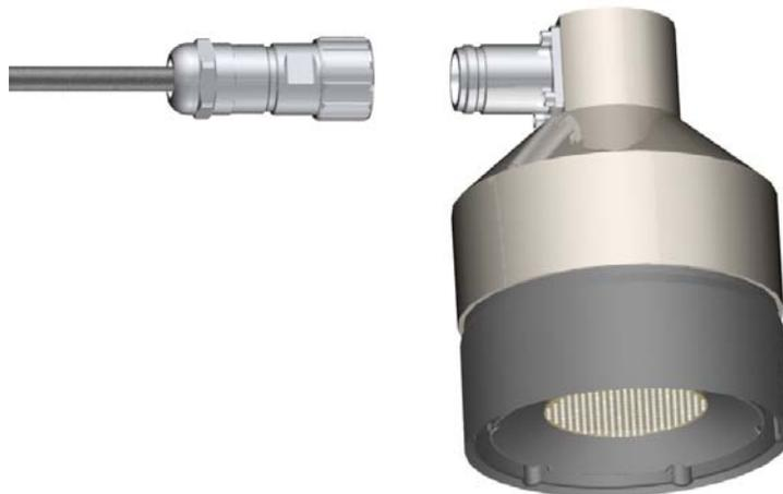
*FIGURE 7. Disconnect Cable from Sensor*
