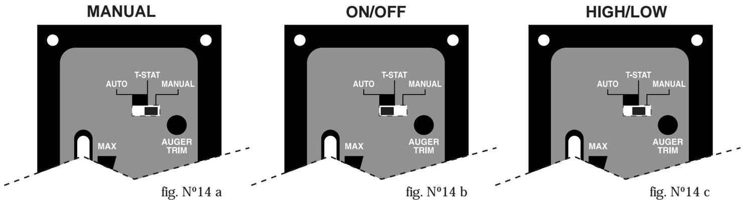
Set damper control rod approximately 1/2" to 3/4" out. This will vary depending on elevation and weather conditions. Observe stove's operation and adjust damper
