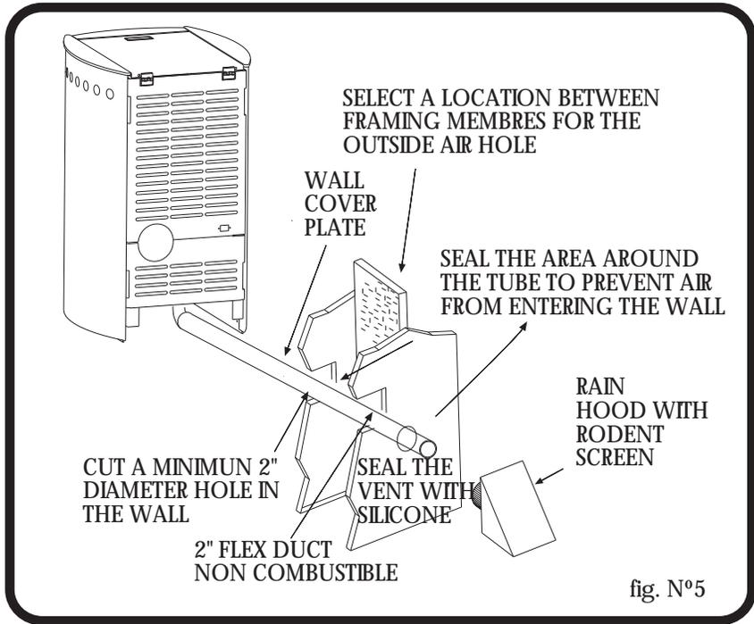
For Mobile home installations only: 2" inside diameter pipe may be used for first 5 feet of combustion air supply run. From 5 to 10 feet use 2 3/4" inside diameter pipe. No combustion air supply may exceed 10 feet.
