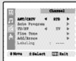
Note: STD, HRC and IRC identify various types of cable TV systems. Contact your local cable company to identify the type of cable system that exists in your particular area.
