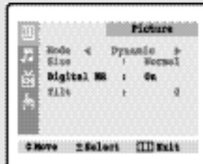
◀ Pressing the **VOL-** or **VOL+** button will alternate between "On" and "Off".
