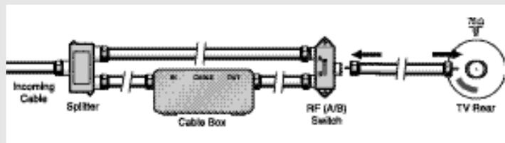
After you've made this connection, set the A/B switch to the "A" position for normal viewing. Set the A/B switch to the "B" position to view scrambled channels. (When you set the A/B switch to "B", you will need to tune your TV to the cable box's output channel, which is usually channel 3 or 4.)
