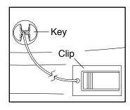
IMPORTANT: In an emergency, the key can be pulled from the console, causing the walking belt to slow to a stop. Test the clip by carefully taking a few steps backward; if the key is not pulled from the console, adjust the position of the clip.
