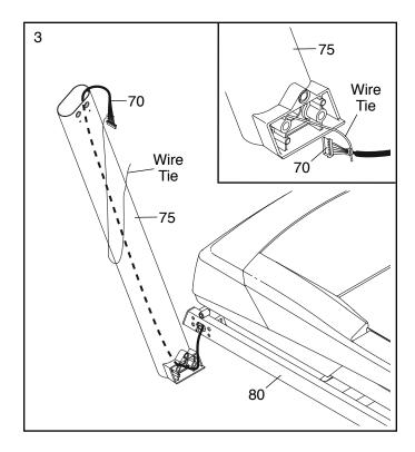
4. With the help of a second person, hold the Left Upright (75) against the Base (80). **Be careful not to pinch the wires.**
