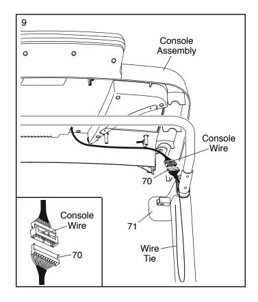
10. Set the console assembly on the Left and Right Handrails (71, 72). **Make sure that no wires are pinched.** Insert the excess Upright Wire (70) into the Left Handrail.
