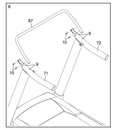
9. With the help of a second person, hold the console assembly near the Left Handrail (71) and the Right Handrail (not shown).
