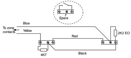
Figure 21 Example: Wiring Two Door Contacts to One FSL Zone.
