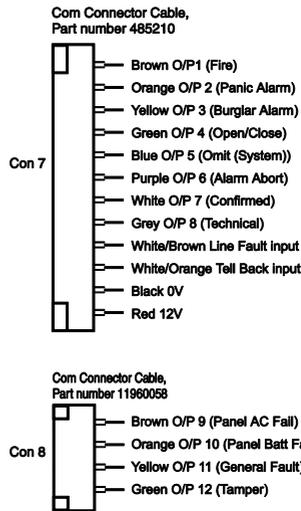
Figure 31 Plug-By Communicator Wiring
