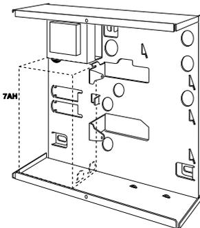
Figure 32 Fitting the Batteries
