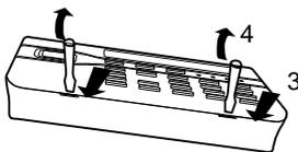
Figure 5 Opening the Keypad
