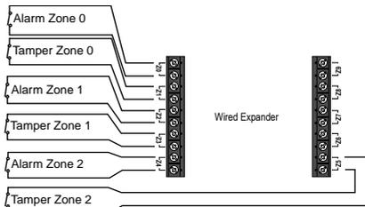
Figure 17 Wired Expander CCL Zone Wiring
