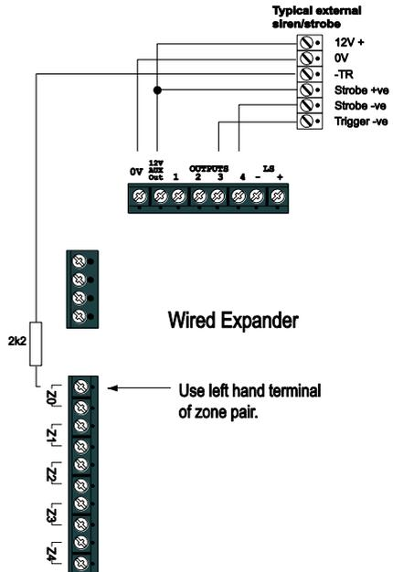
Figure 27 Wiring -TR from External Sounder to a FSL Zone on the Expander.
