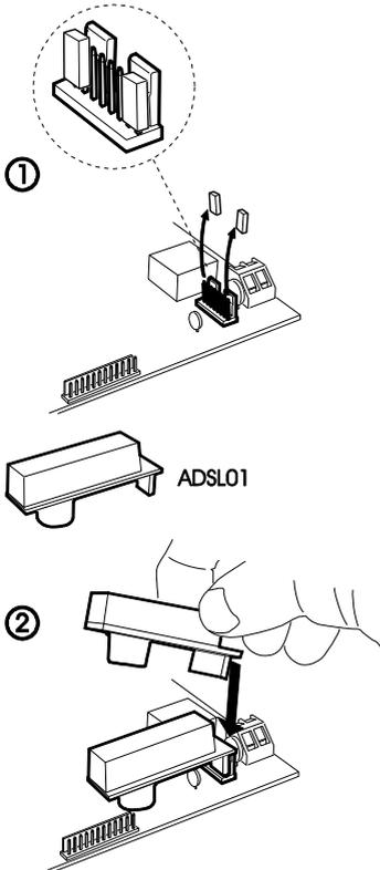
Figure 30 Fitting the ADSL01 Filter.
