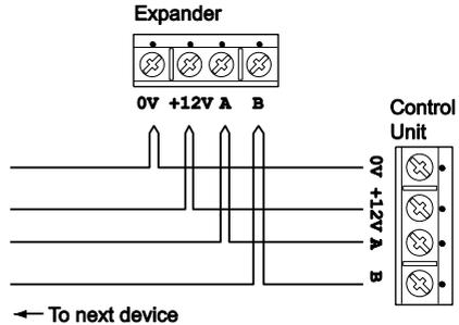
Figure 14 Wiring Expanders
