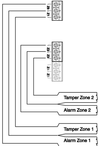
Figure 16 Control Unit CCL Zone Wiring
