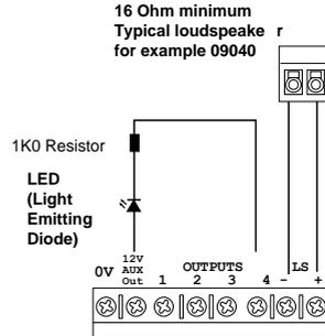
Figure 24 Using Wired Expander Outputs.
