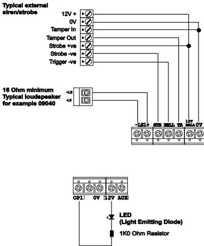
Figure 23 Connecting Wired Peripherals
