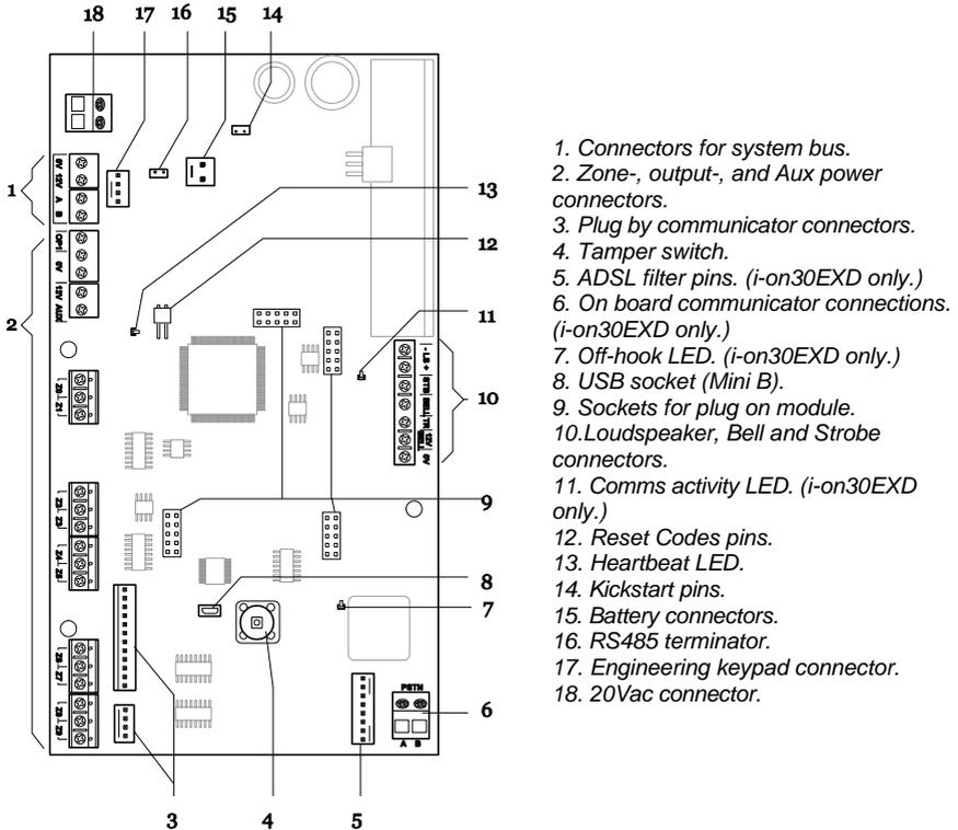
Figure 2 Control Unit Printed Circuit Board
