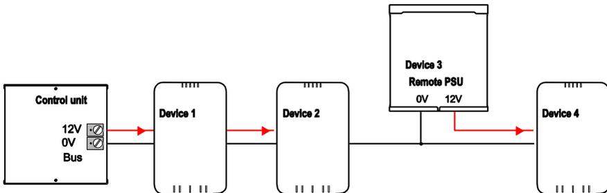
Figure 11. Connecting Remote Power Supply Units
