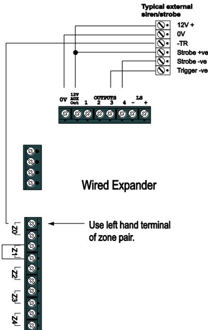
Figure 26 Wiring -TR from External Sounder to a - 4 wire CC Zone on the Expander.
