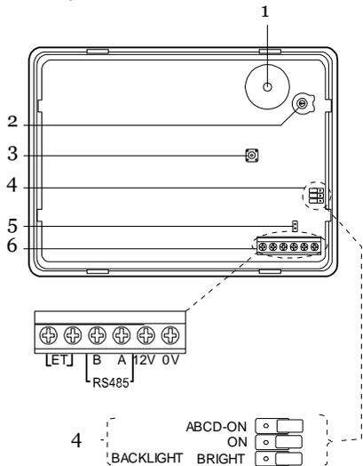
Figure 7 Keypad PCB
