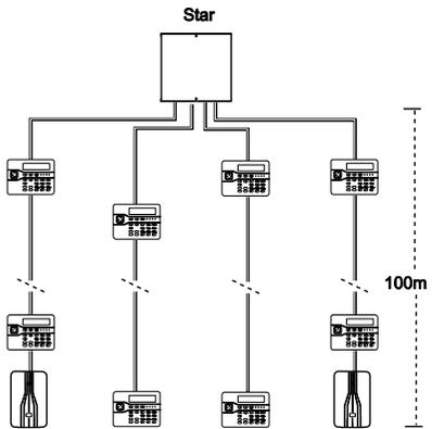
Figure 10 Bus Wiring Configurations
