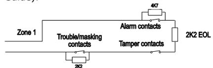
Figure 22 Example: Wiring a Trouble/Masking Zone, 3 Resistor Method.
