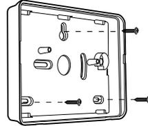
Figure 12 Screw Keypad Back Box to Wall
