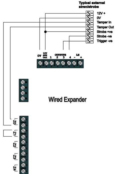
Figure 25 Wiring External Sounder to Expander
