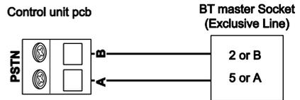
Figure 29 Connecting the Internal Communicator
