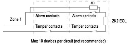
Figure 20 Wiring Two Detectors per Zone FSL.
