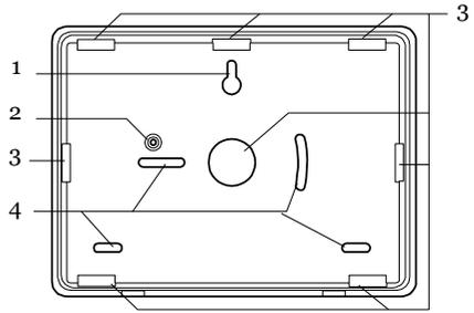
Figure 6 Keypad Rear Housing
