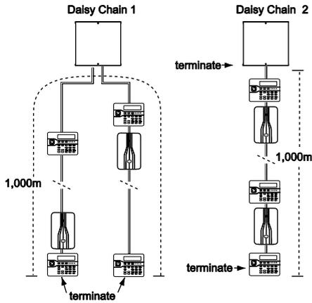
devices either in daisy chain (serially), or in star (parallel) configuration at the control unit connector.
