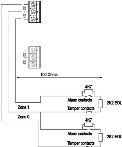
Figure 18 FSL Zone Wiring - Control Unit
