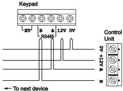
Figure 13 Connecting a Keypad to the Bus
