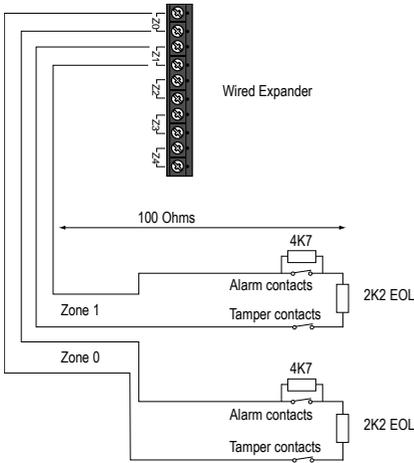
Figure 19 FSL Zone Wiring - Expander
