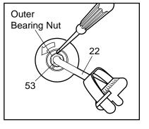
screwdriver in one of the slots in the outer bearing nut. Tap the screwdriver with a hammer to turn the Outer Bearing Nut counterclockwise until the arms are no longer loose. Do not overtighten the Outer Bearing Nut. When the Outer Bearing Nut is properly tightened, retighten the Hex Jam Nut.
