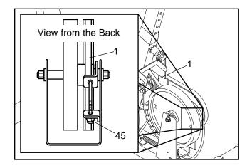
Next, locate the Drive Belt (1). To tighten the Drive Belt, turn the 3/8" Locknut (47) slightly; be careful not to overtighten the Drive Belt. When the Drive Belt is properly adjusted, reattach the left side shield, flywheel cover and left pedal.
