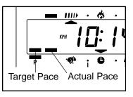
the display. The left column will show one bar, showing that the target pace is 5 mph (8 kph). The right column will show your actual pedaling pace. Adjust your pedaling pace until only one bar appears in the right column. Each time the target pace changes during the program, adjust your pedaling pace to keep both columns at the same height.
