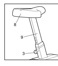
several turns to loosen it. Next, pull back the Seat Knob, slide the Seat Post (9) to the desired height, and release the Seat Knob. Move the Seat Post up or down slightly until it locks into place. Turn the Seat Knob clockwise to tighten it.
