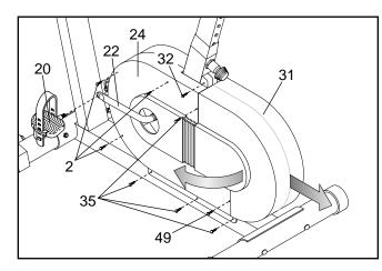
Cover (31) must be removed. Using an adjustable wrench, turn the Left Pedal (20) clockwise and remove it. Next, remove the indicated Screws (2, 32, 35, 49). Turn the left arm of the Crank (22) to the position shown and slide off the Left Side Shield and the Flywheel Cover.
