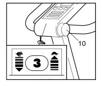
of the console will show which resistance level you have selected. Level 0 is the easiest level, and level 10 is the most challenging.
