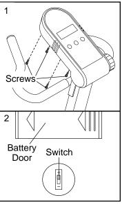
switch up or down to change the unit of measurement. Reattach the console with the four screws.
