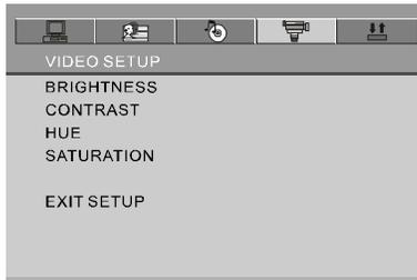
3 Press the DOWN button to highlight the desired option. Press ENTER or RIGHT to select the choices of that option appear.
