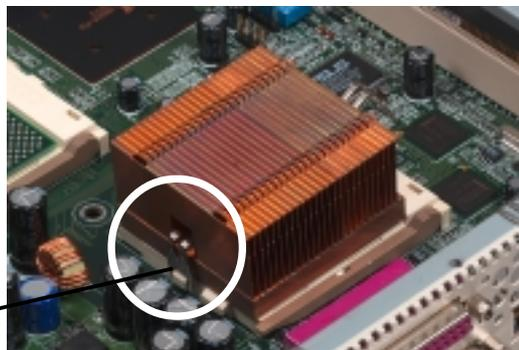
2. Use a flat screwdriver to hook the other end of the retaining clip to the protruding tab at the back of the CPU socket.
