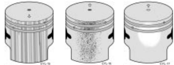
Carbon scoring produces soft-edged grooves on the exhaust side of the piston. Piston rings are still free in the grooves.
