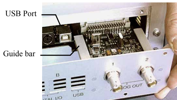
Fig. 12: Installing the DAC board
