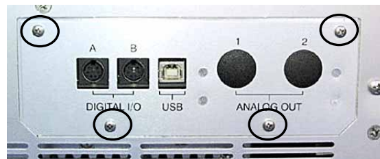
Fig. 11: Screws on the access panel
