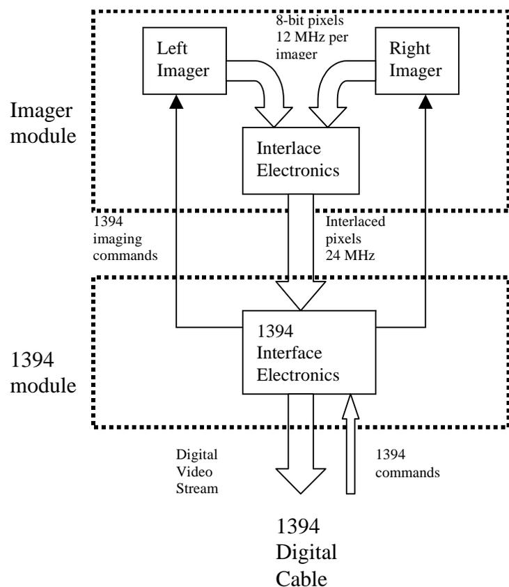
**Figure 3-2 Schematic of the STH-DCSG-C electronics.**
