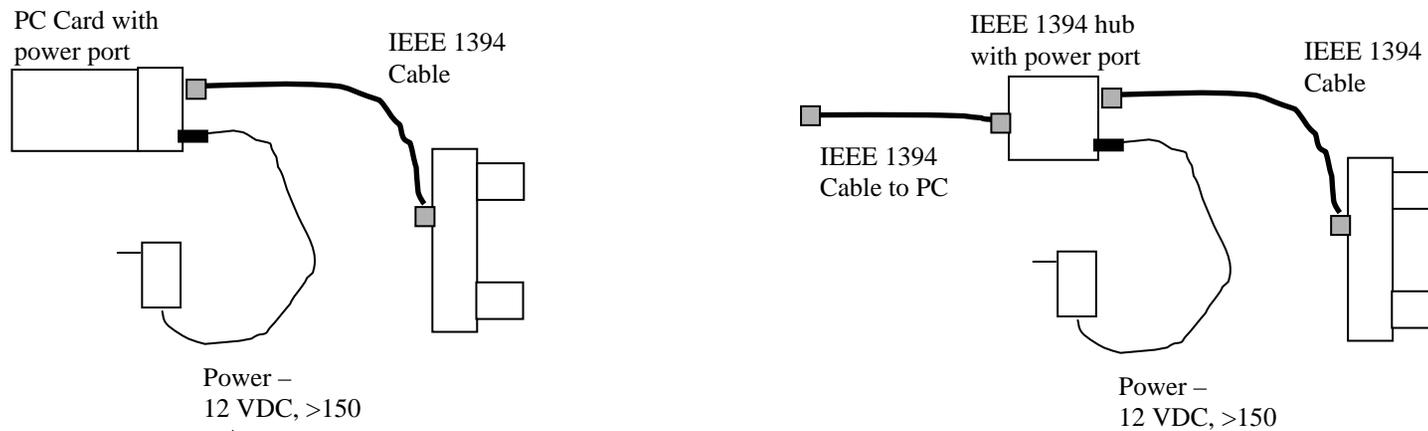
**Figure 5-1 External power supply connections. On the left is power supplied to a PC Card with a power port. On the right, power is supplied through a hub with a power port. Power should be 7 to 16 VDC, at > 1.5 W. Check the PC Card or hub for the type of power connector.**
