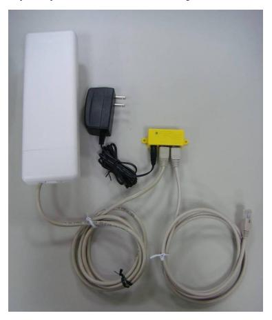
Notes: Use **Reset button** on POE injector. Push continually the reset button of POE injector about 5 ~10 seconds to reset the configuration parameters to factory defaults.
