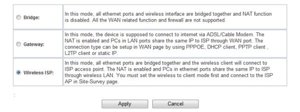
In **Wireless ISP** mode, all ethernet ports are bridged together and the wireless client will connect to ISP access point. The NAT is enabled and PCs in ethernet ports share the same IP to ISP through wireless LAN. You must set the wireless to client mode first and connect to the ISP AP in Site-Survey page.
