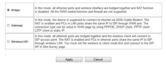
In **Bridge** mode, all ethernet ports and wireless interfaces are bridged together and NAT function is disabled. All the WAN related function and firmware all not supported.
