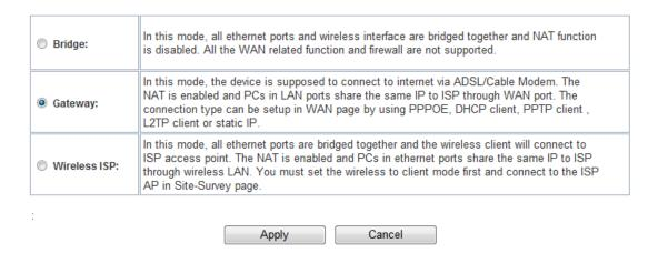
In **Gateway** mode, the device is supposed to connect to internet via ADSL/Cable modem. The NAT is enabled and PCs in LAN ports shard the same IP to ISP through WAN port. The connection type can be setup in WAN page by using PPPOE, DHCP client, PPTP client, L2TP client or static IP.
