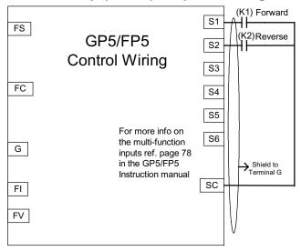
This configuration is used when the Start/Stop is via an external source such as a PLC or relay. It can also be used with a maintained switch when it is desirable to have the inverter restart on the return of power. It should not be used where the safety of personnel might be threatened by the restart of the machine.
