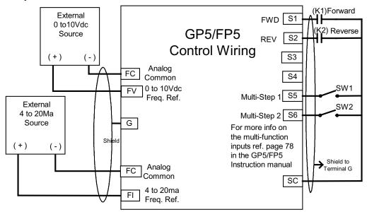
This configuration is generally used when the inverter is controlled via a remote source such as a PLC. It can also be used with a maintained switch when it is desirable to have the drive restart on restoration of power. It should not be used where the safety of the attending personnel might be threatened by automatic restart. Up to three speeds can be selected by using the switches SW1-SW2 to select the desired speed.
