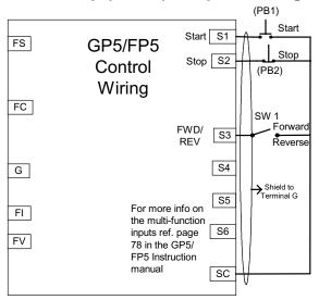
This mode is commonly used when a inverter is replacing existing equipment such as an across the line starter and the application requires minimal to no speed changes.
