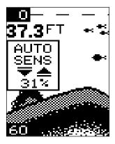
After you've adjusted the unit to the desired sensitivity level, press the ON/CLEAR key to clear the display. If you wait a few seconds, it will automatically clear.
