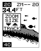
This means the Magna III is tracking the bottom in a zoom window, always keeping it on the display.
