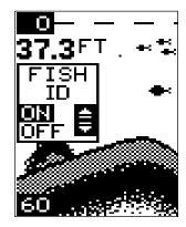
The Fish ID feature can't be used when the Magna III is in the manual mode. If you turn the automatic feature off, the Fish ID feature will automatically be turned off, also.
