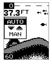
Pressing the ON/CLEAR key also clears it. To turn the automatic feature on again, repeat the above steps, except this time press the up arrow key.
