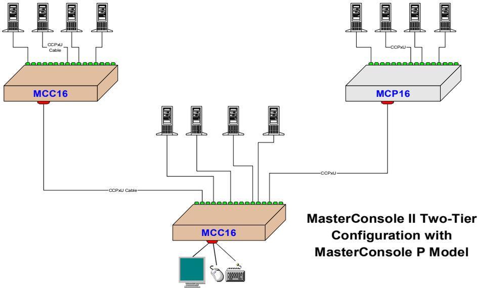
Figure 27. Two-Tier Configuration with MasterConsole P Model
