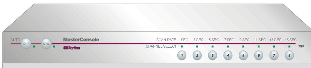
Figure 6. MasterConsole II Front Panel
