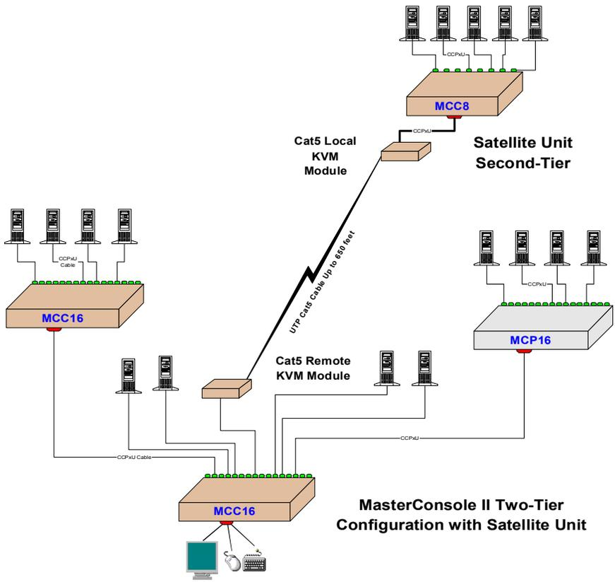
Figure 28. Two-Tier Configuration with Satellite Unit
