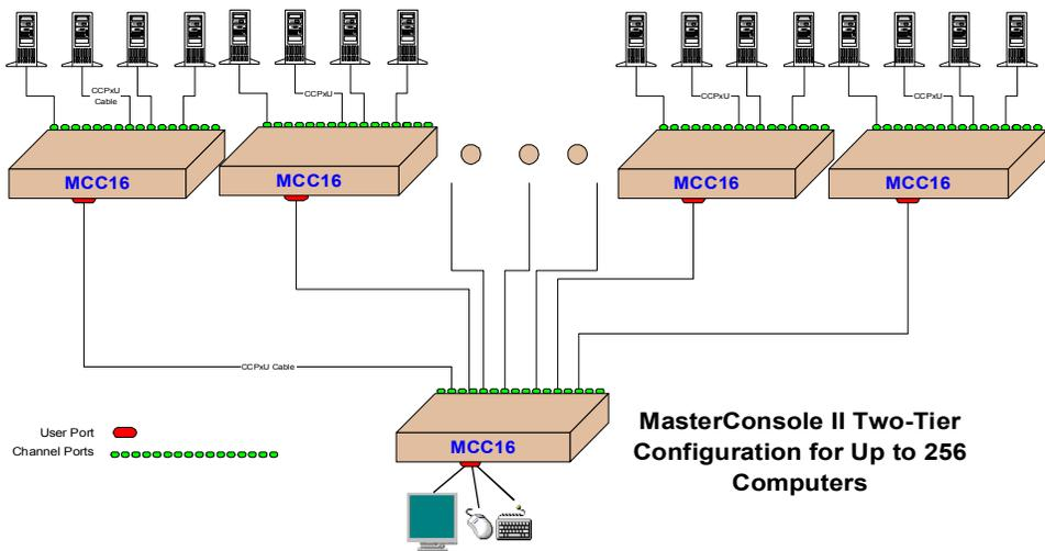
Figure 26. Two-Tier Configuration of up to 256 Computers
