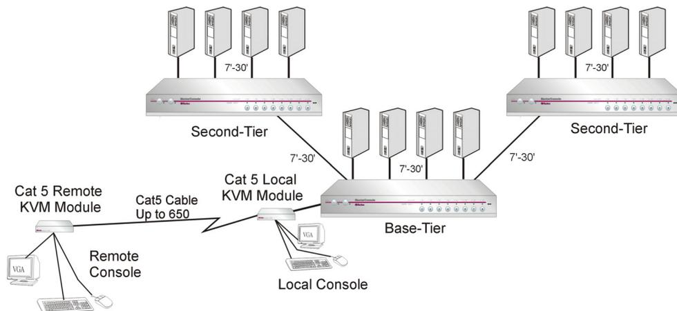
Figure 12. Two-Tier Configuration (With optional Remote Access Kit)
