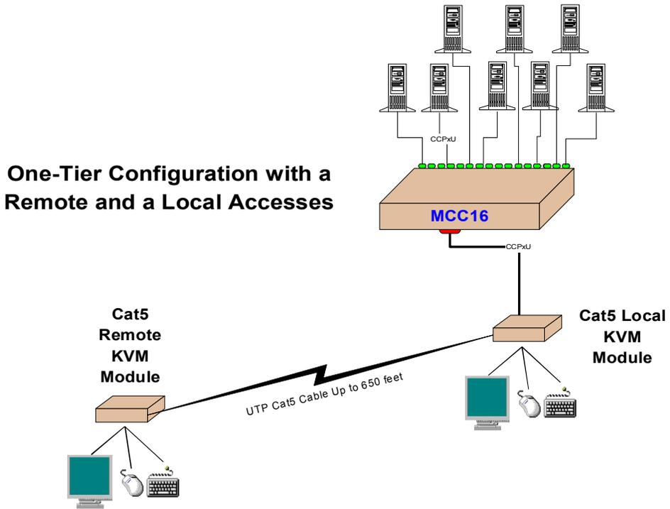
Figure 25. One-Tier with Remote Access Kit
