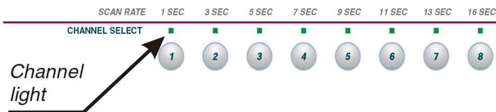
Figure 7. MasterConsole II Front Panel (Channel lights)
