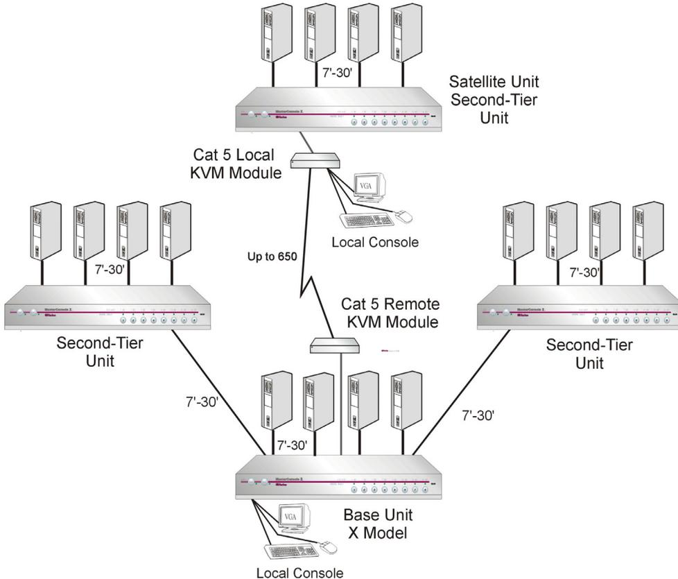
Figure 23. Two-Tier Configuration with Satellite Unit
