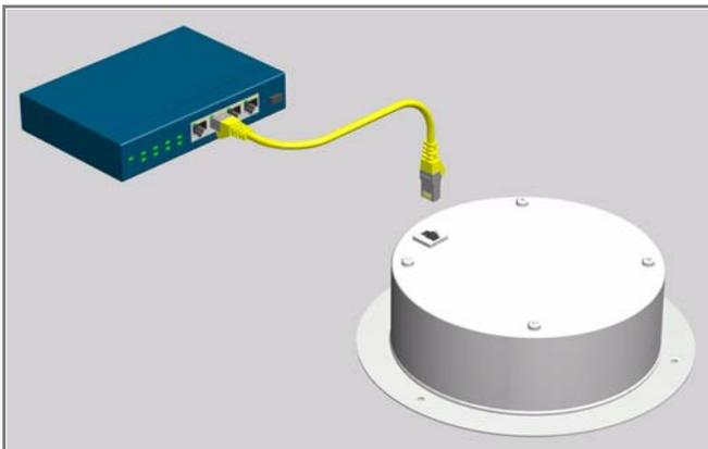
**Figure 2-2. PoE Injector**
