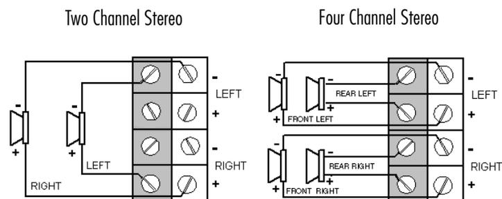
**NOTE:** For bridged two channel operation as shown in this diagram, connect right channel RCA cables to the front inputs of the amplifier, and left channel RCA cables to the rear inputs of the amplifier. For summed subwoofer applications, connect RCA cables per the input jack marking.
