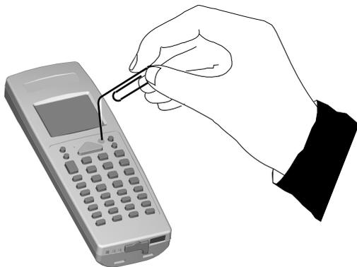
To activate the reset button insert a blunt-ended object into the hole. The reset function will delete all RAM data.
