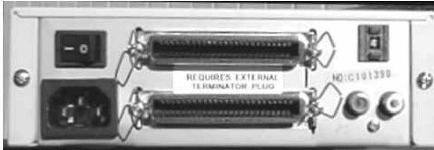
Plug the end of the SCSI cable into the TOP port of the DVD player. (The other end of the cable is connected to the card you installed in your computer.)
