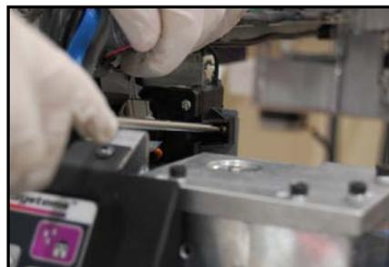
4. Remove the locking bracket holding the unit to the side plate. Use pliers to remove the bracket from the side of the print engine.
