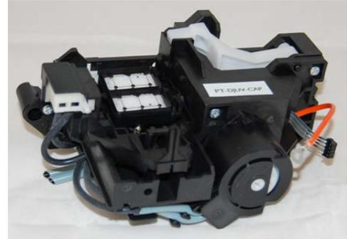
The Capping Station is mounted to the printer with 5 Philips head screws (4 hold it in place + 1 for the orange ground wire). There is also 1 small electrical connector that needs to be disconnected.
