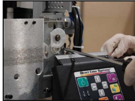
5. Disconnect the electrical cable that goes to the motor. Do not leave the gender changer connected to the capping station. Leave it connected to the wire that is attached to the printer.
