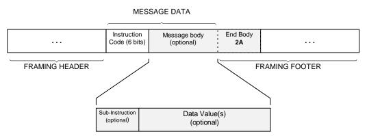
In this protocol, the first byte of the message data is referred to as the *instruction code*, which ranges in value from **00** to **20**. Normally if there is a reply, it will contain the same instruction code as the host message.
