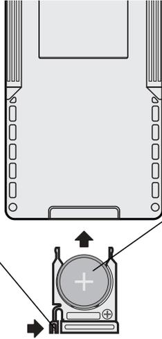
2. Remove the old battery and insert a new CR2025 button cell Lithium battery in the battery compartment tray, + side up.
