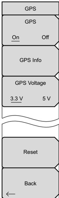
**GPS:** Press this submenu key to turn GPS on or off.
