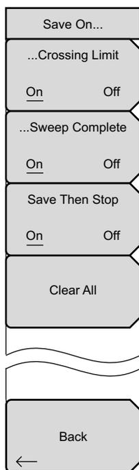
In Spectrum Analyzer mode, this menu is used to auto save measurements to internal memory after:
