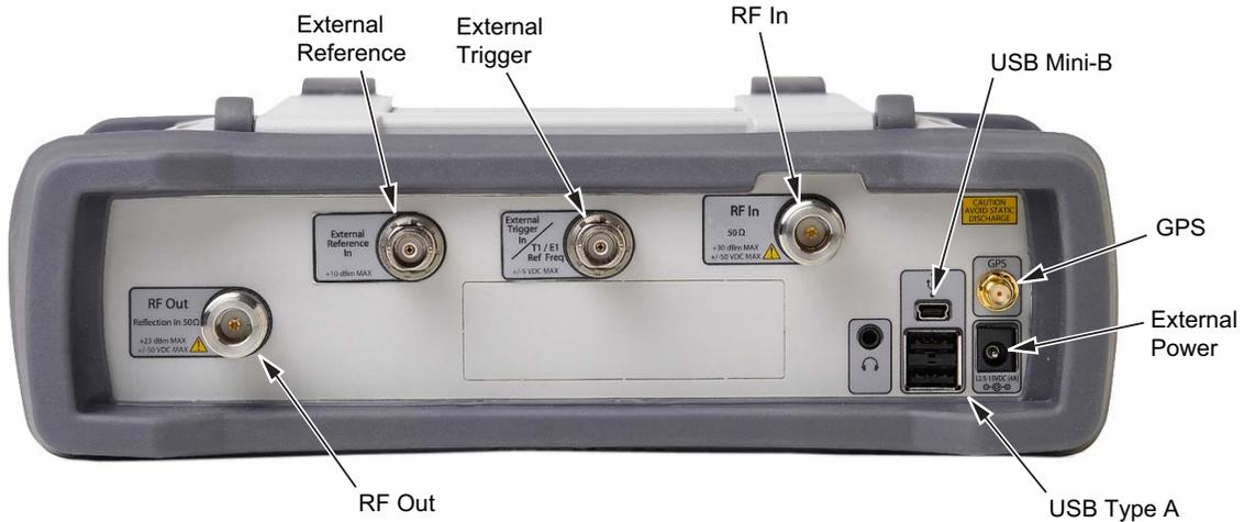
**Figure 2-7.** S332E Test Panel Connector
