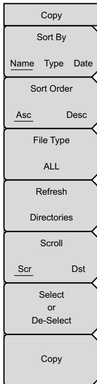
This menu and dialog box is used to copy folders and files. Select folders or files with the **Up/Down** keys, the scroll wheel or the touch screen.
