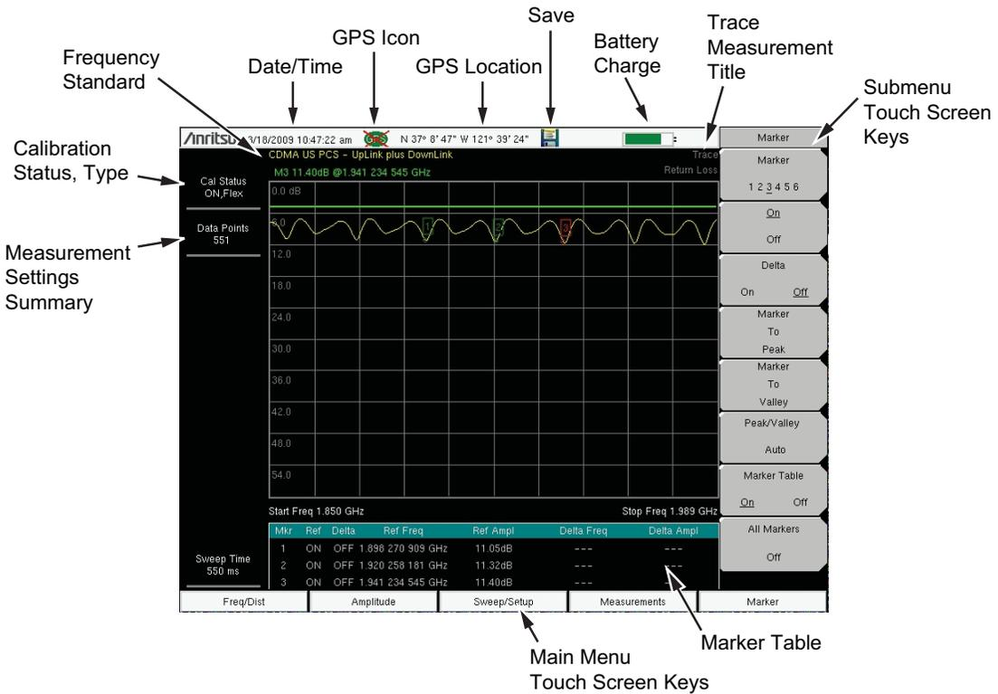
Figure 2-5. Cable & Antenna Analyzer Return Loss Measurement Display
