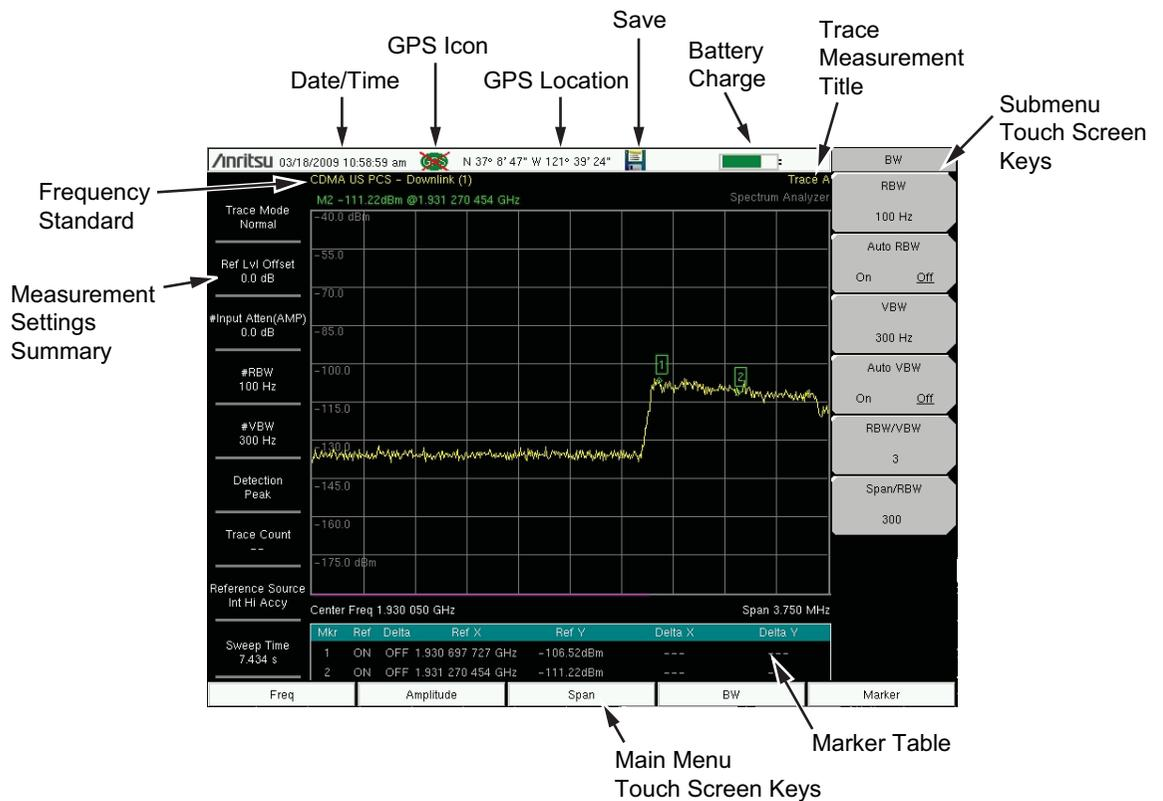
Figure 2-6. Spectrum Analyzer Display (S332E and S362E only)
