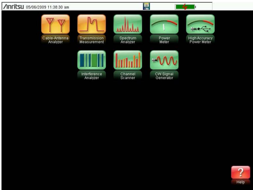
**Figure 2-2.** Menu Key Screen, Icons for Installed Measurements
