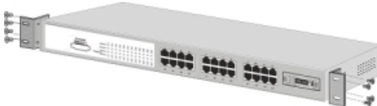
Figure 2-4. Attach mounting brackets with screws
