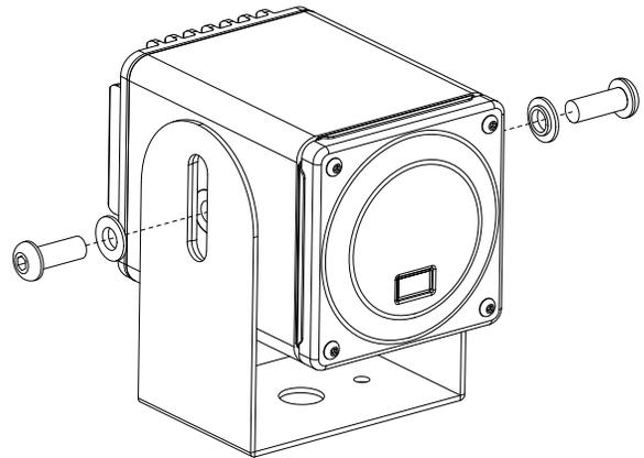
3. Secure the loudspeaker to the U-bracket using the two 3/8-16 screws and two shoulder washers included with the MUB-MM4XP. The shoulder washers should be placed between the screws and the outside of the U-bracket, with the shoulder oriented toward the loudspeaker. Do not yet tighten the U-bracket screws.
