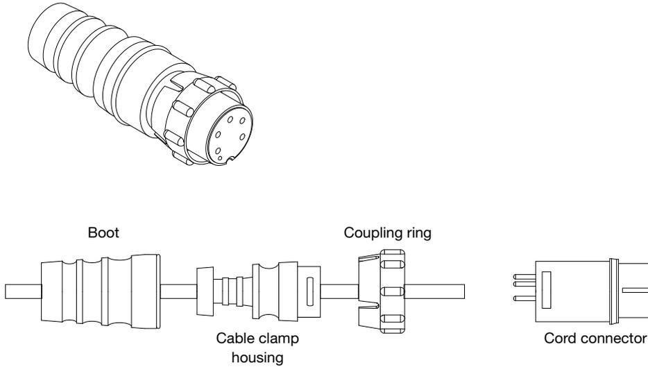
Disassembled EN3 5-Pin Female Cable Mount Connector
