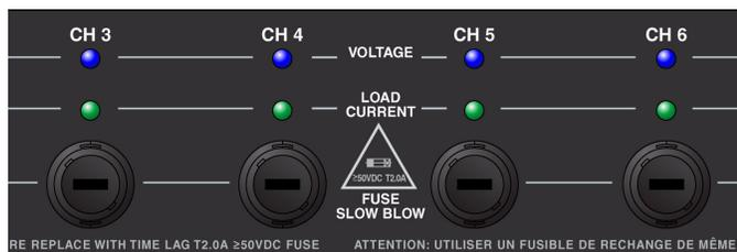
MPS-488 Channel LEDs and Fuses
