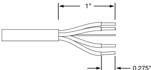
3. Solder the five exposed conductors to the five pins on the EN3 cord connector using the following wiring scheme.
