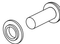
**CAUTION:** Make sure to use the shoulder washers. They insulate the MM-4XP from the U-bracket and mounting surface, eliminating grounding and differential problems.
