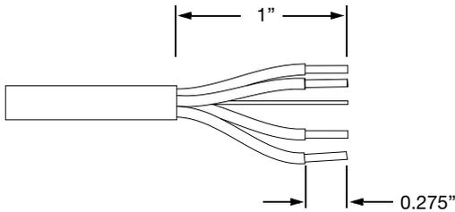
2. Insert the five exposed conductors into the five cable holes in the Phoenix connector using the following wiring scheme.
