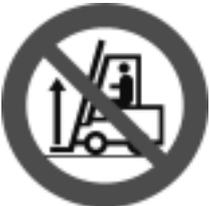
This pictogram shows that no horizontal transport devices must be placed under this frame section, such as pallet lifters or the forks of fork lift trucks. It is also forbidden to place lifting devices for transport and storage under this frame element.
