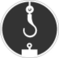
This pictogram shows where the AHU must be lifted and is positioned on the support beam.
