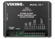
are also stored in non-volatile memory. All programming is done with a local touch tone phone. Up to three ES-1s can be programmed simultaneously if they will be sharing all the same programming codes and parameters. Entry logging is possible with the ES-1's log bus data output.
