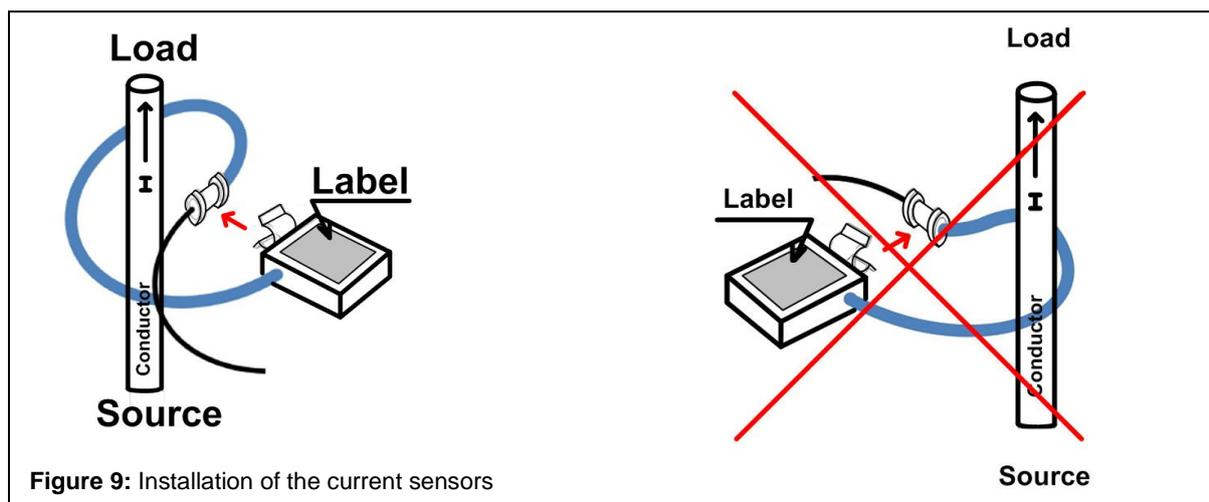
The label on the coil must be aligned in such a way that it points towards the consumer. This ensures the correct direction of current flow through the coil.
