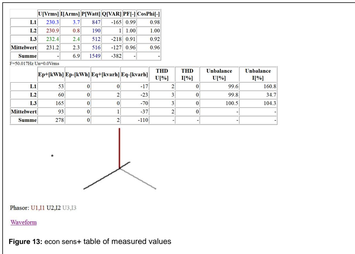
The following are displayed: the voltages of the phases L1, L2, L3, the corresponding currents, as well as the active and the reactive power per phase and the “power factor” (for pure sinusoidal alternating currents, this is synonymous with the familiar cos phi).
