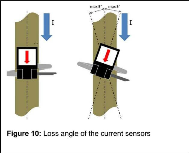
In the case of loss angles  $> \pm 5^\circ$ , the relative error of measurement is also greater and consequently also the relative deviation of the measured current and the calculated parameters (e.g. power).
