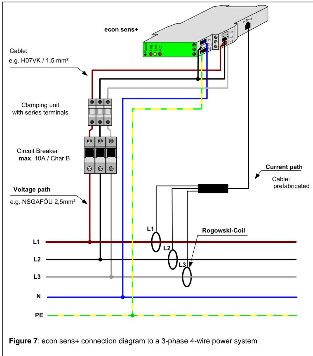
The phases L1, L2 and L3 of the voltage path must be protected by means of automatic circuit breakers to prevent the system from being damaged in the event of a short circuit. A B6 (max. B10) automatic circuit breaker is recommended. For safety reasons it is preferable to use a short-circuit-proof conductor (NSGAFÖU) in front of the circuit breakers.
