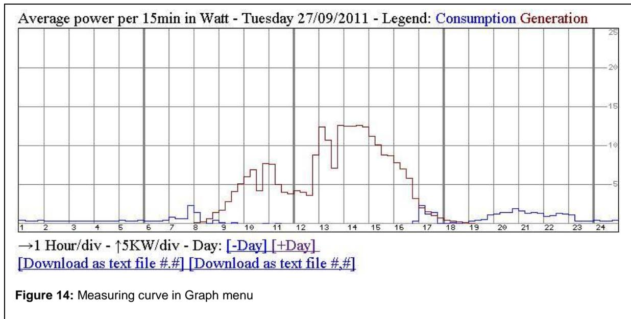
The sum of the power/energy from the three phases is shown over a certain period of time. Using the – *period* and + *period* buttons next to the X-axis label you can toggle through the measuring curves step by step (e.g. every day of a month).
