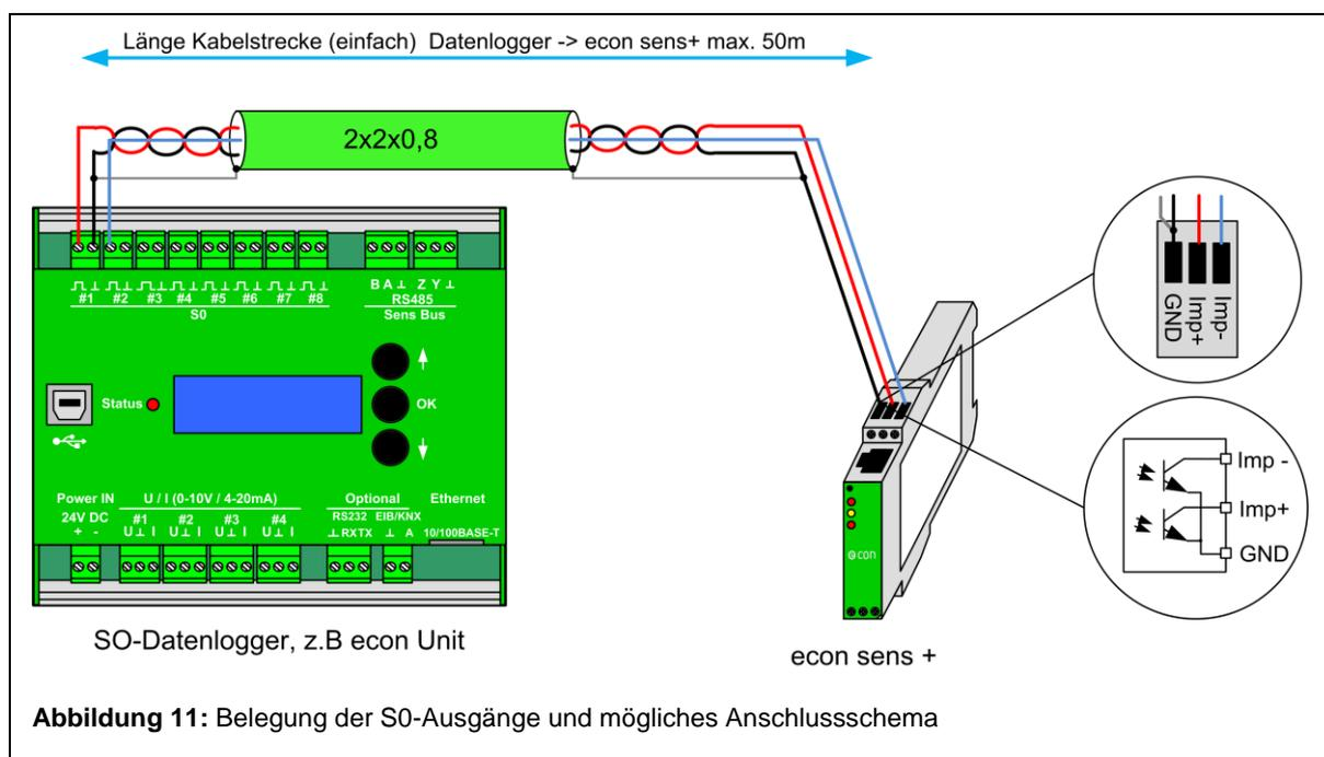
The distance between the data logger and the econ sens + may be amount to max. 50 meter. When connecting a cable, a shielded cable is recommended \*, as Belden YE00820. For shorter distances an unshielded cable can be used.
