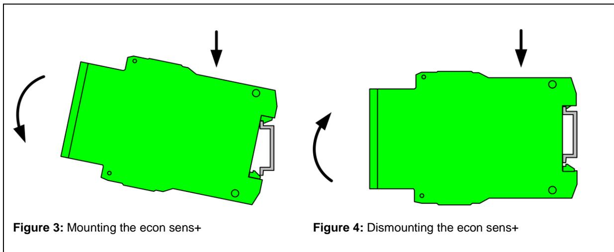
The device is dismantled as shown in Fig. 6. Press the device downwards using light pressure and then pivot it upwards.
