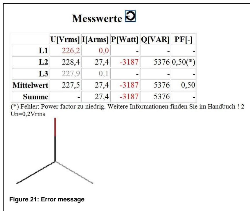
In the table of measured values it can be seen that the power factor of phase 2 has dropped below 0,71 and the phase shift between U2 and I2 in the graphic "Phasor" has 120°. This is a typical error pattern for the above-named Installation errors.
