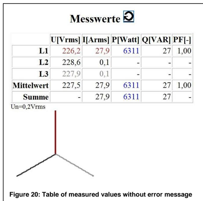
General, it is assumed that all measurement coils were installed correctly, and the measured load has a power factor of >0.71 (phase shift between U and I <45 °). Then the table of measurements in Figure 20 is shown. In this example, a load of about 6 kW measured at L1, L2 and L3 are unloaded.
